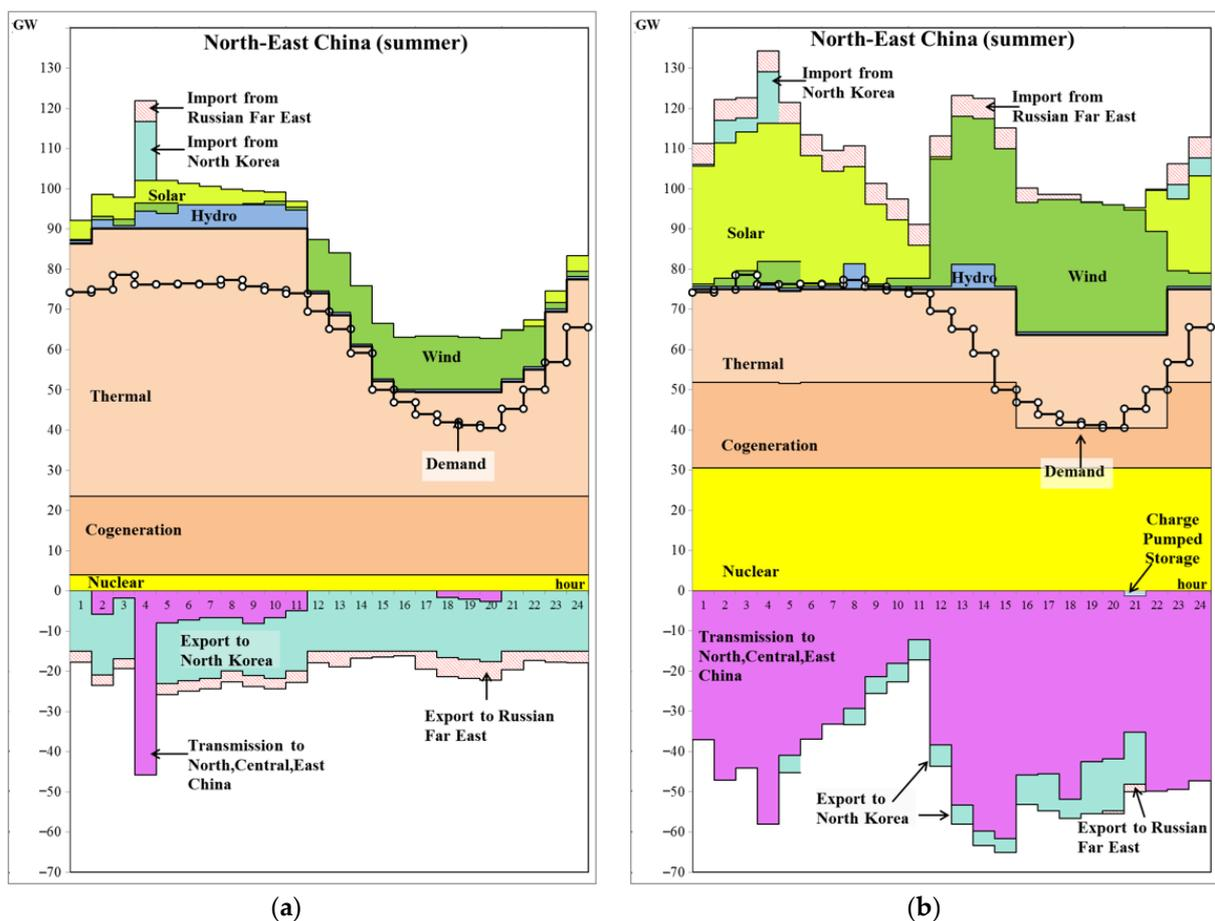
**Figure 10.** North-East China's EPS operating modes (dispatching) within the NEA ISPG. Source: compiled by authors based on computing results. (a) No CO<sub>2</sub> emission tax. (b) CO<sub>2</sub> emission tax in USD 90/ton.
