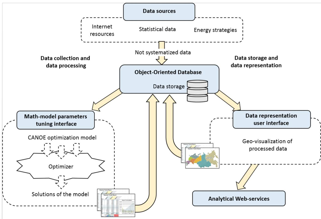
**Figure 1.** Structural and functional diagram of CGIS. Source: Author's original figure.
