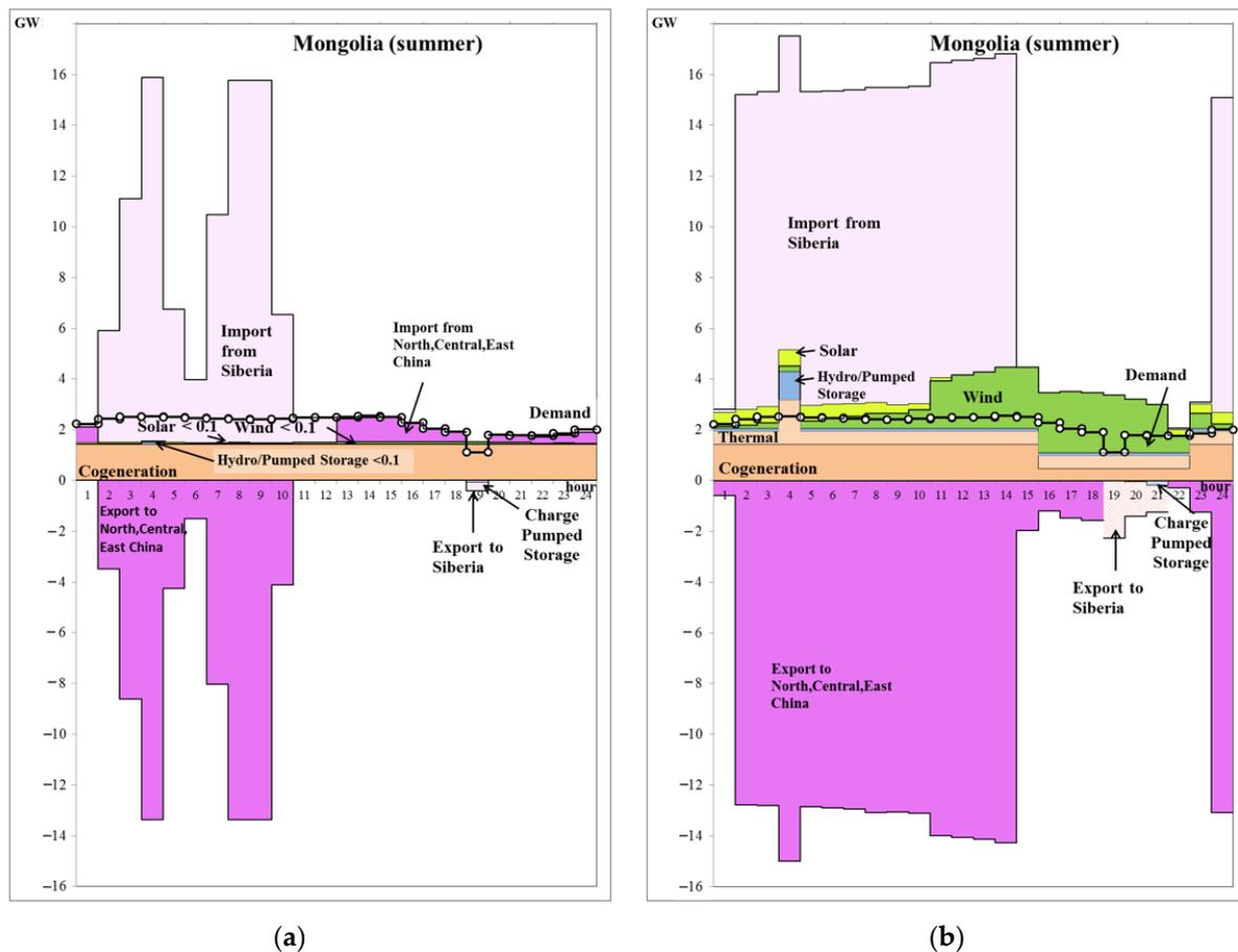
**Figure 9.** Mongolia's EPS operating modes (dispatching) within the NEA ISPG. Source: compiled by authors based on computing results. (a) No CO<sub>2</sub> emission tax. (b) CO<sub>2</sub> emission tax in USD 90/ton.
