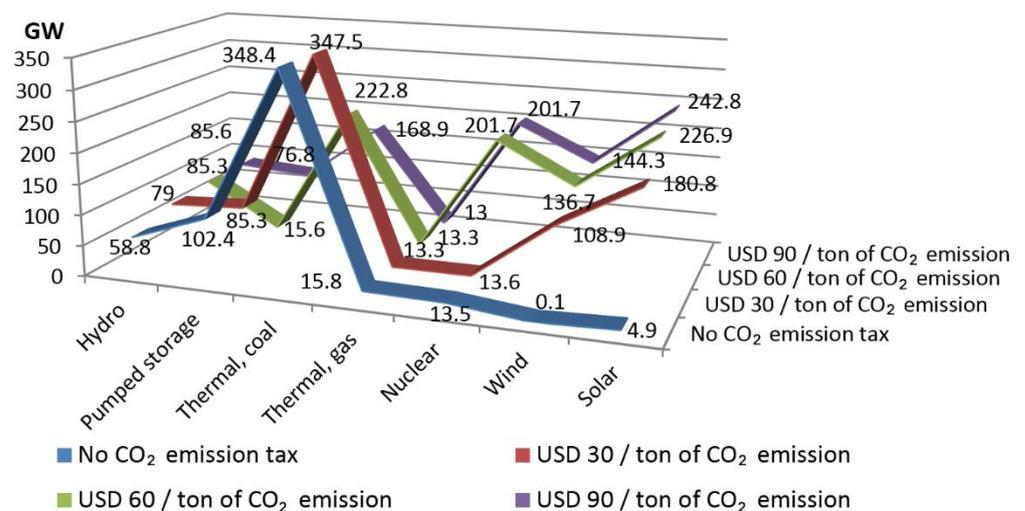
**Figure 3.** Capacity additions by type of power plants and level of CO<sub>2</sub> emission tax, power system interconnection scenario. Source: calculated by authors.
