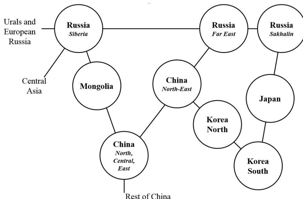
**Figure 2.** The diagram of the prospective interstate power grid in North-East Asia. Source: Author's original figure.
