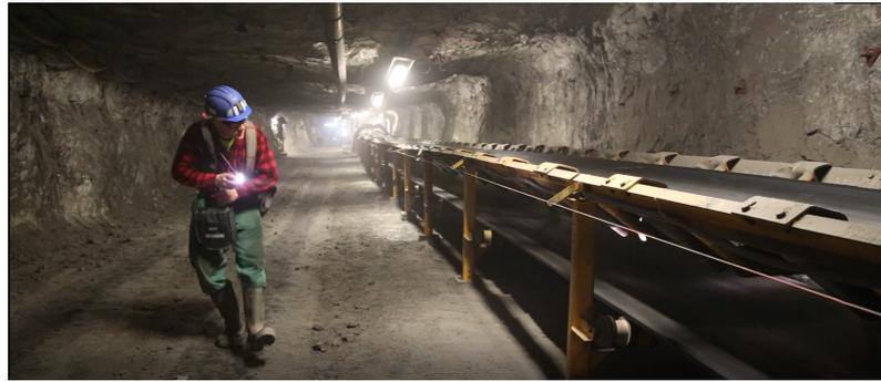
**Figure 1.** Conveyor belt route inspection in traditional form.
