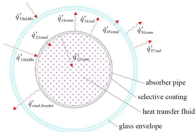
**Figure 7.** One-dimensional steady-state energy balance of SPTC [21].
