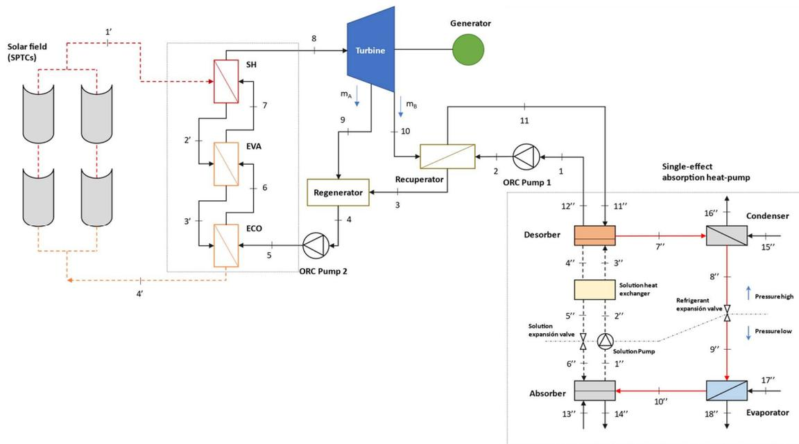
Figure 5. Case 5: CCHP with single-pressure ORC regenerative recuperated superheated cycle (1P REG + REC + SH).
