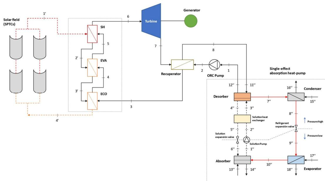
**Figure 4.** Case 4: CCHP with single-pressure ORC recuperated superheated cycle (1P REC + SH).
