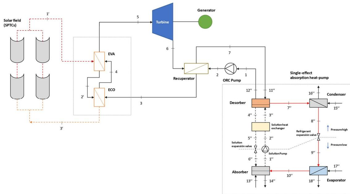
**Figure 3.** Case 3: CCHP with single-pressure ORC recuperated cycle (1P REC).
