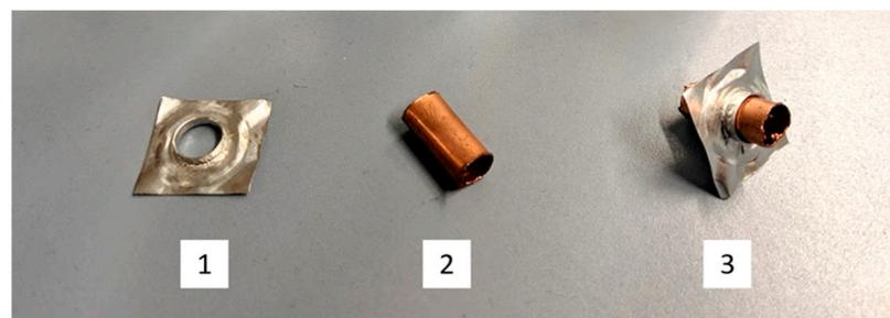
**Figure 2.** Photograph of metallic (1: aluminum, 2: copper, 3: copper and aluminum) samples which were used for material compatibility experiments.
