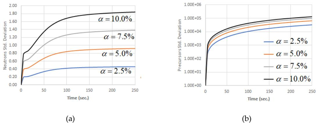
Figure 2. (a) Deviations in power due to random parameters. (b) Deviations in delayed precursors due to random parameters.
