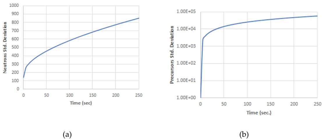
**Figure 3.** (a) Deviations in neutronic power due to noise; (b) deviations in delayed precursors due to noise.
