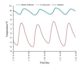
Figure 26. The temperature of Rural House 2 after the renovation.
