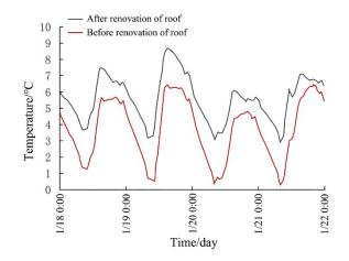
Figure 16. The simulated temperature of the master bedroom before and after renovation of the roof.
