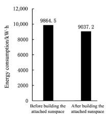
Figure 15. The annual cumulative heating energy consumption before and after building the sunspace.
