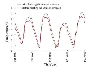
Figure 14. The simulated temperature of the master bedroom before and after building the sunspace.
