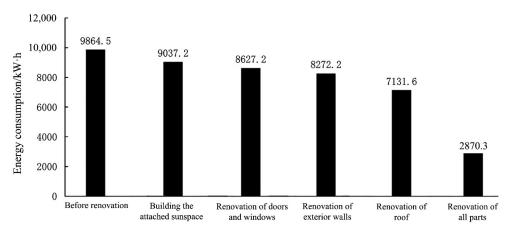
Figure 24. Effects of different renovation measures on heat energy consumption.
