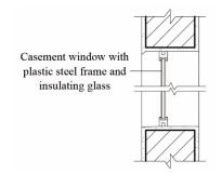
Figure 32. Replacing with a new window.
