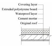
Figure 28. Outdoor roof insulation.
