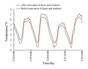
**Figure 20.** The simulated temperature of the master bedroom before and after renovation of doors and windows.
