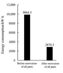
Figure 23. The annual cumulative heating energy consumption before and after renovation of all parts.
