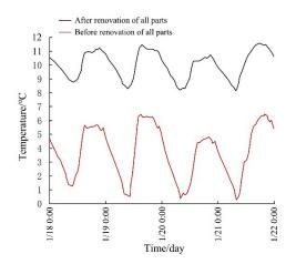
Figure 22. The simulated temperature of the master bedroom before and after renovation of all parts.
