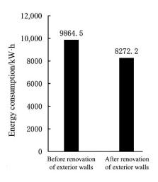
**Figure 19.** The annual cumulative heating energy consumption before and after renovation of exterior walls.
