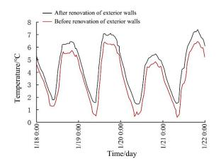
**Figure 18.** The simulated temperature of the master bedroom before and after renovation of exterior walls.
