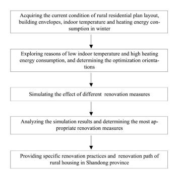
Figure 7. The flow for transforming a rural house.
