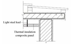
Figure 29. Indoor insulation ceiling.
