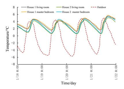
Figure 5. Outdoor and indoor temperature test results of rural houses.
