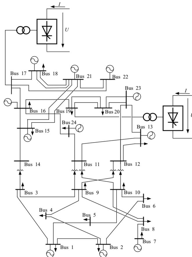
Figure 1. Improved IEEE reliability test 79 system.
