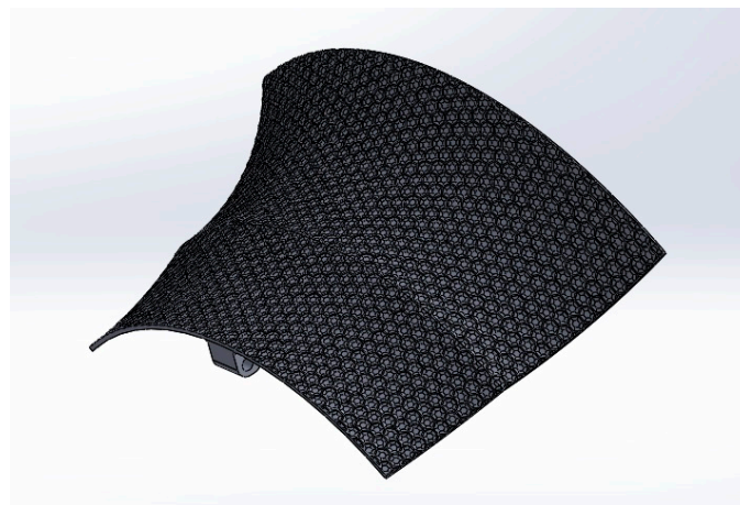
Figure 17. View of the reflector model with a diffusing macrostructure.
