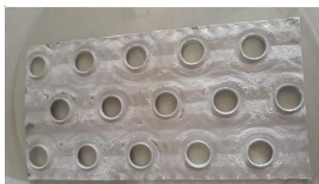
**Figure 9.**  $\text{Al}_2(\text{SO}_4)_3$  can be coated as uniform layers as thin as  $15 \text{ mg/cm}^2$  on a plate of Al.
