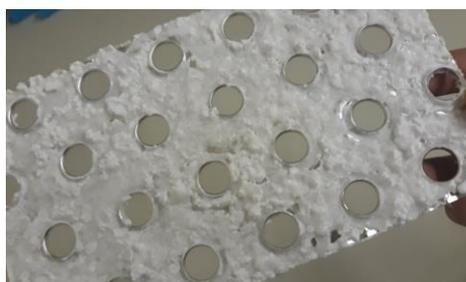
**Figure 15.** Composite  $\text{MgSO}_4$ -hydrate/PVOH with improved stability.
