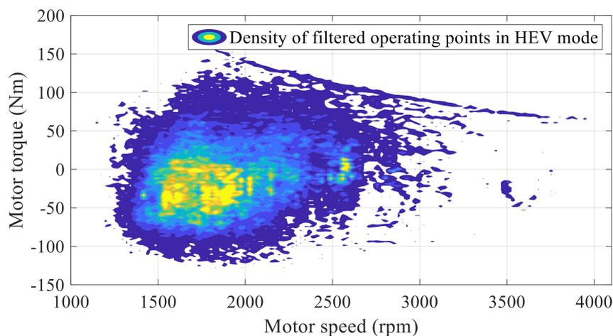
Figure 17. Density of Operating Points of the Motor.
