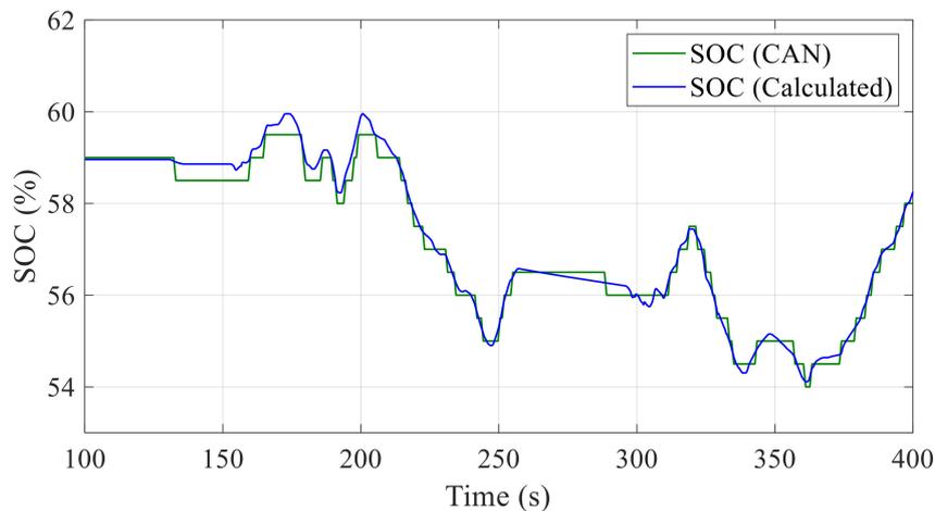
Figure 7. Comparing SOC Signal from CAN with SOC Calculated.
