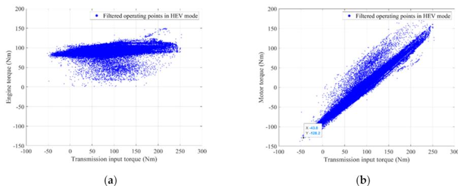
**Figure 14.** Engine and Motor Torque According to the Transmission Input Torque: (a) Engine Torque in Hybrid Mode, (b) Motor Torque in Hybrid Mode.
