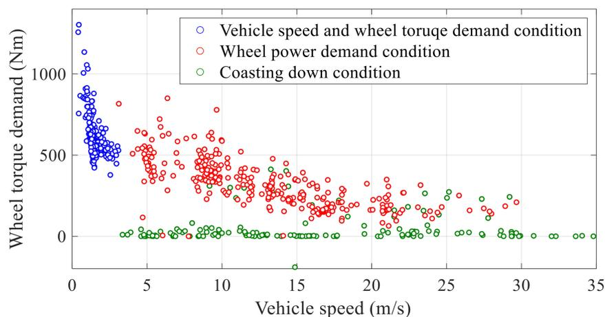
Figure 9. “Engine on” Conditions with Filters Applied.
