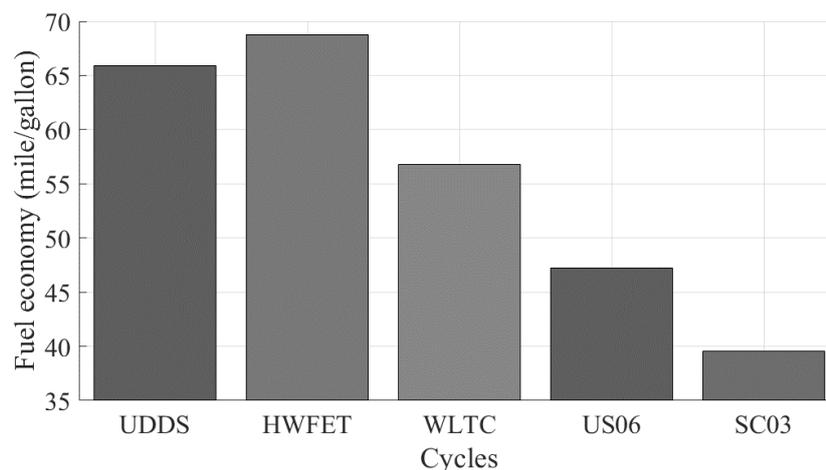
**Figure 4.** Fuel Economy according to Cycles with Hot Test: Urban Dynamometer Driving Schedule (UDDS), Highway Fuel Economy Test (HWFET), Worldwide Harmonized Light Vehicles Test Cycles (WLTC), High Acceleration Aggressive Driving Schedule (US06), Use of Air Conditioning Driving Schedule (SC03).
