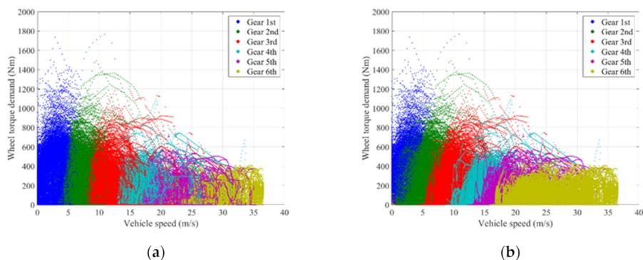
Figure 13. Estimated Shifting Map of Ioniq HEV: (a) Up Shifting Map, (b) Down Shifting Map.
