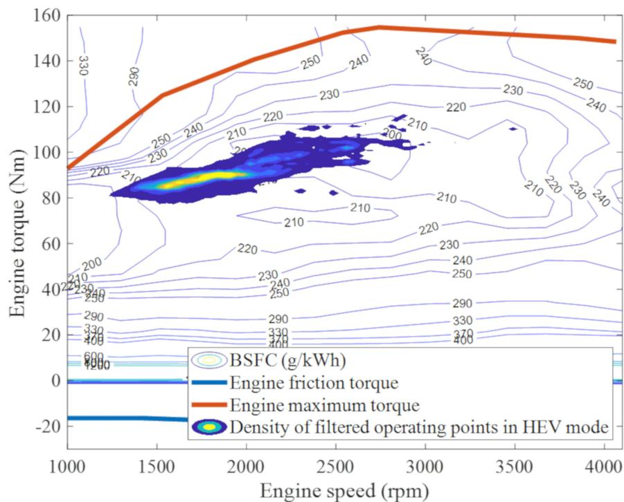
Figure 16. Density of Operating Points of the Engine with BSFC.
