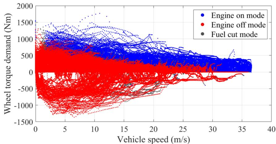
Figure 8. All Operating Points According to the Engine Status.
