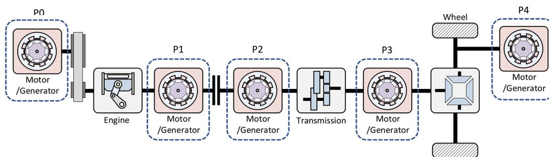
Figure 1. Parallel Hybrid System Configuration.
