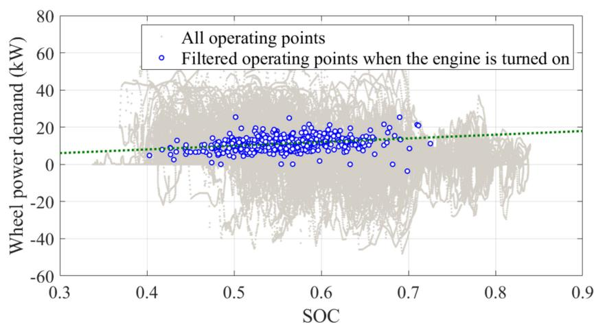
**Figure 11.** Operating Points When the Engine is Turned on According to the SOC.
