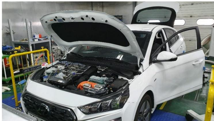
**Figure 3.** Dynamometer Test of Ioniq HEV.
