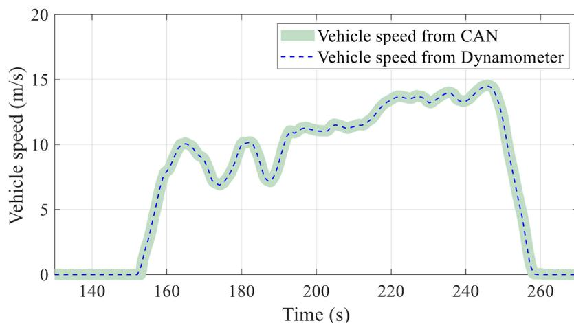
**Figure 5.** Signal Alignment of Vehicle Speed Signals.
