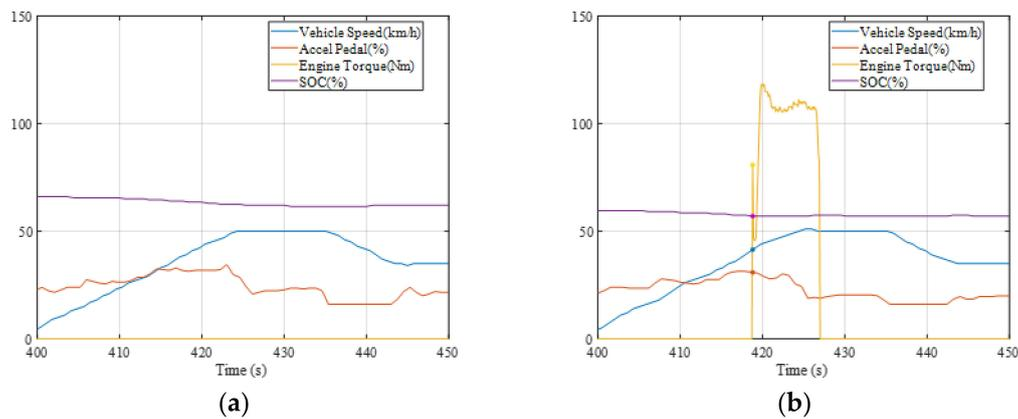
**Figure 10.** Dynamometer Test Results with NEDC Cycle: (a) NEDC Cycle Test Results with High SOC, (b) NEDC Cycle Test Results with Low SOC.
