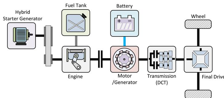
Figure 2. Powertrain System Configuration of Ioniq HEV.
