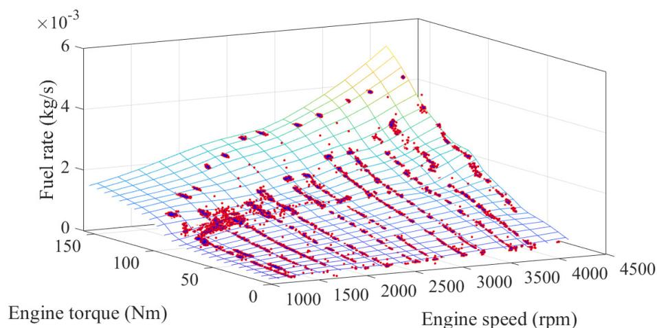
**Figure 15.** Engine Fuel Map Based on Load Tests.
