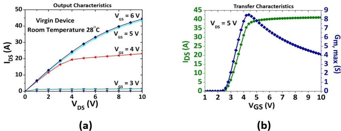
**Figure 2.** Representative of commercialized GaN cascode 650 V power switch virgin electrical characteristics: (a) output characteristics and (b) transfer characteristics.
