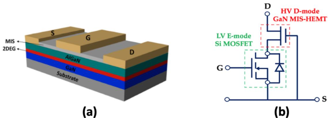
**Figure 1.** (a) Most favorable Gallium Nitride (GaN) Metal-Insulator-Semiconductor High-Electron-Mobility-Transistor (MIS-HEMT) structure and (b) a schematic diagram of the GaN cascode configuration, where high voltage D-mode GaN MIS-HEMT and normally-off low voltage Si-MOSFET are in a series of connection.
