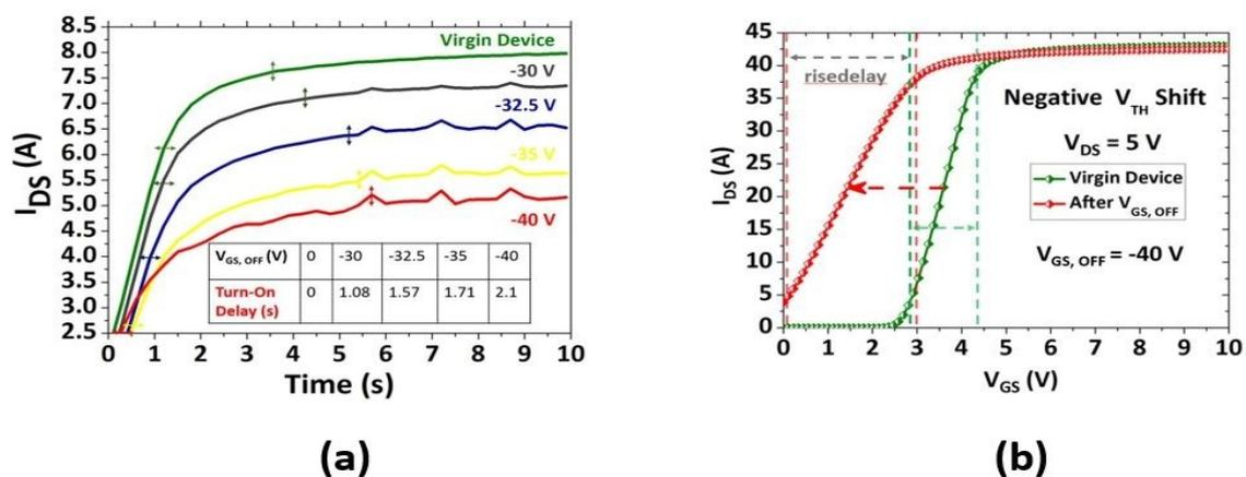
**Figure 7.** (a) Turn-On delay (Gate-Lag) effects under high  $V_{GS, OFF}$  pulsed stress and (b) Rise-Time  $t_r$  delay and  $V_{TH}$  shift for high  $V_{DS}$  and  $V_{GS, OFF}$ .
