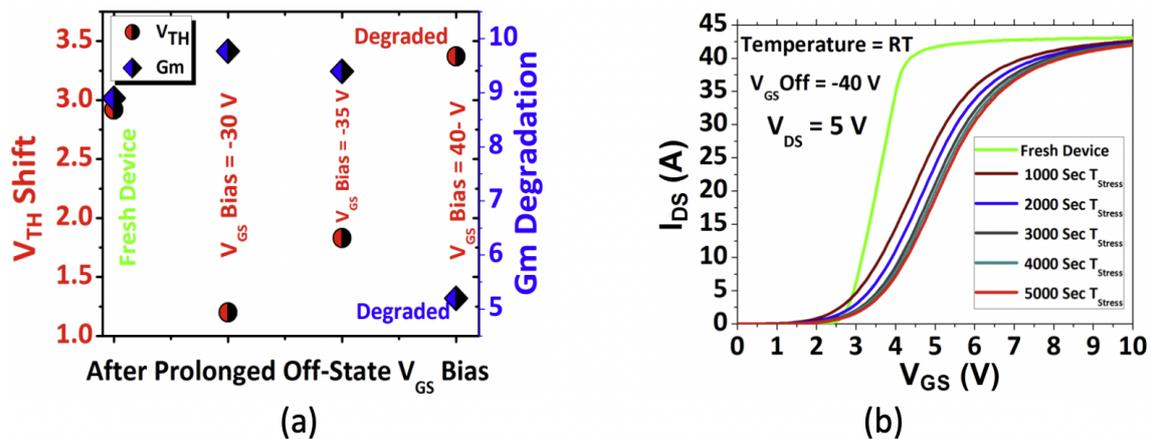
**Figure 8.** Results of prolonged off-state gate stress bias on cascode 650 V power switch: (a) transfer characteristics of prolonged off-state gate bias ( $-40$  V) and (b) threshold voltage shift and transconductance degradation after prolonged (5000 s) off-state  $V_{GS}$  Bias.
