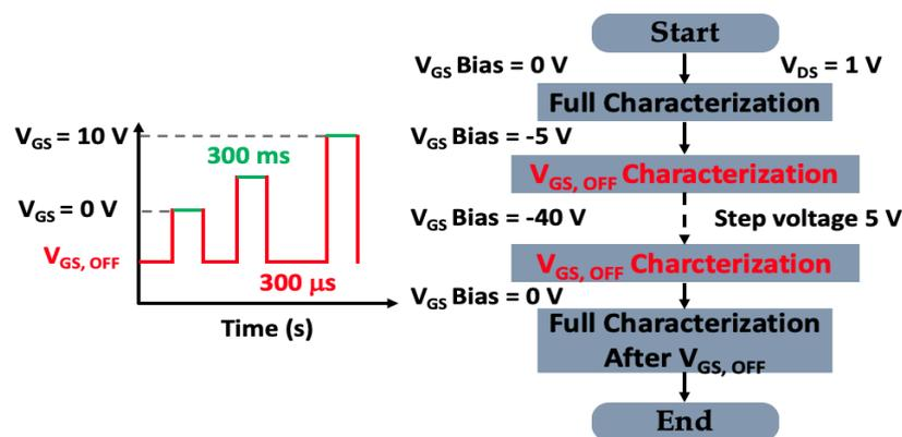
**Figure 3.** Schematic stress waveform and flow chart of control voltage pulsed ( $V_{GS, OFF}$ ) bias stress experiment.
