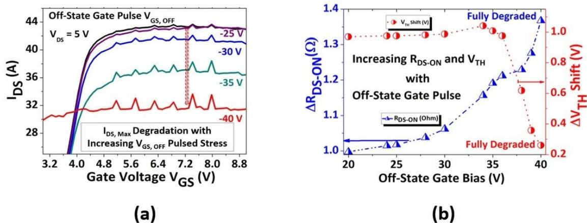
**Figure 6.** Results of pulsed off-state gate stress bias on cascode 650 V power switch: (a)  $I_{DS}$  degradation for high-stress off-state gate bias values and (b)  $\Delta R_{DS-ON}$  degradation and  $\Delta V_{TH}$  shift for high stress off-state gate pulsed bias.
