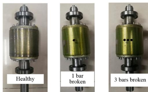
**Figure 10.** Photos of the Rotors with Holes.
