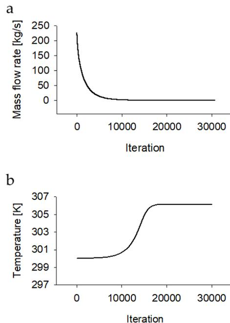
**Figure S2.** Monitoring the stabilization of temperature and mass flow rate during the iterative calculation.
