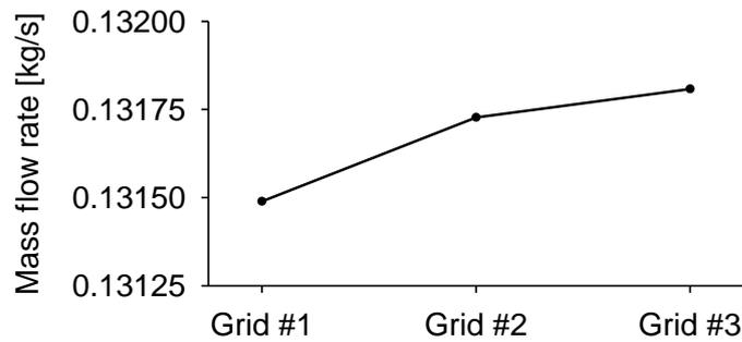
**Figure S1.** Grid independence test.
