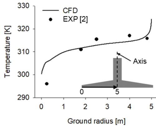
**Figure S3.** Comparison of the temperature profiles between the CFD results and experiment results [2].
