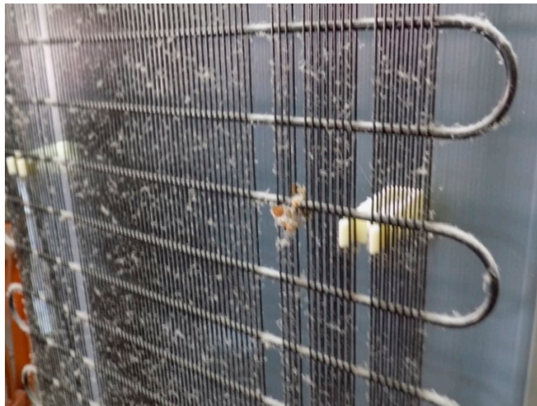
Figure 10. Typical fouling in a condenser.
