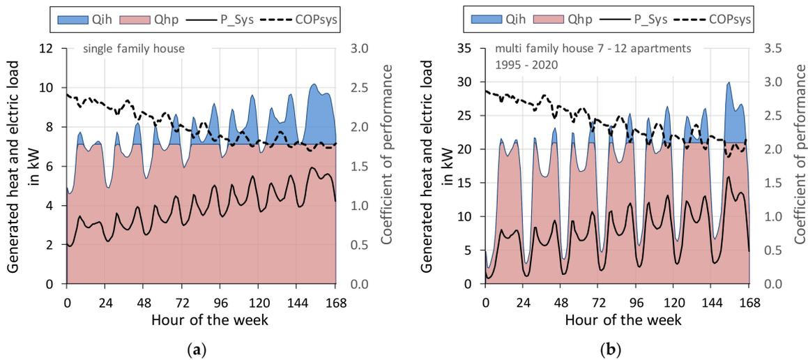
**Figure 5.** Generated heat, electric load and COP of an air source heat pump system in a single family house before 1979 (a) and a multi family house of the building age class 1995–2020 (b).
