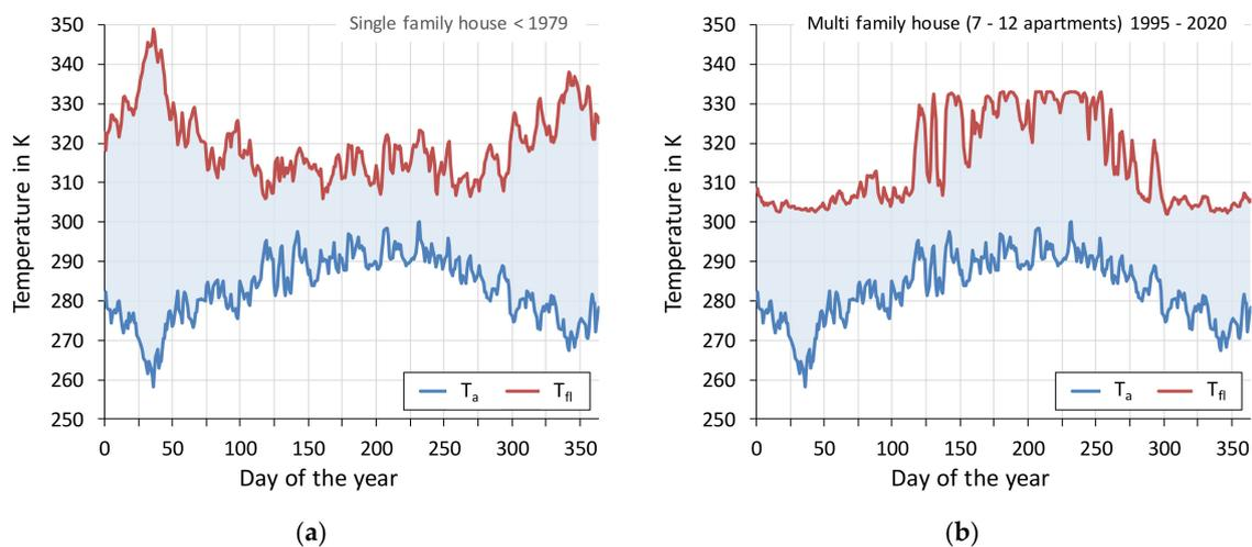
**Figure 3.** Ambient air temperature ( $T_a$ ) and floor temperature ( $T_{fl}$ ) of an air source heat pump in a single family house of the building age class before 1979 (a) and a multi-family house with seven to 12 apartments of the building age class 1995 to 2020 (b).
