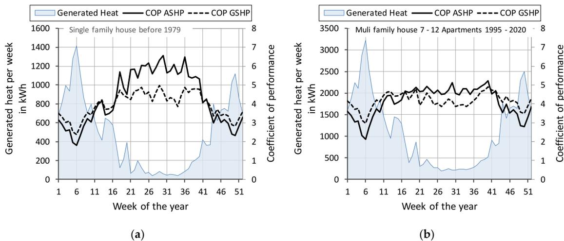
**Figure 4.** Comparison of the COP and the generated heat of an air source heat pump and a ground source heat pump for a single family house before 1979 (a) and a multi-family house of the building age class 1995–2020 (b).
