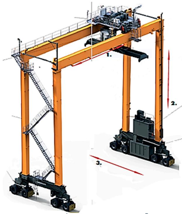
**Figure 1.** Directions of motions of rubber tire gantry crane (RTGC) (1-Trolley, 2-Hoist, 3-Gantry).
