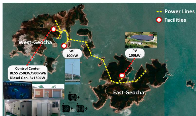
**Figure 1.** Isolated microgrid on Geocha Island, South Korea.
