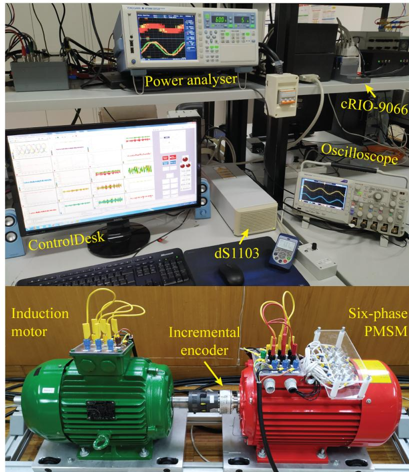
Figure 14. Experimental setup.
