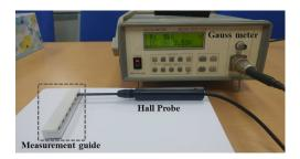
Figure 11. Gauss measurement of the magnet surface.
