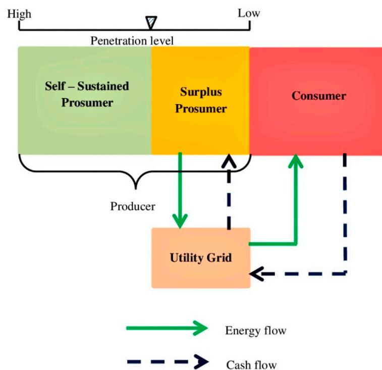
Figure 1. Conventional peer-to-grid (P2G) trading.
