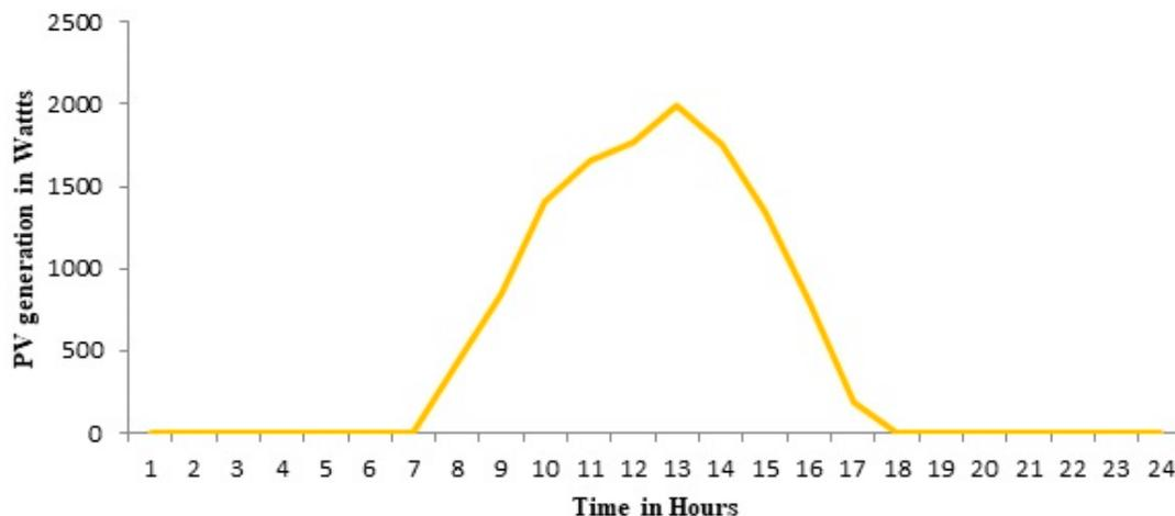
Figure 5. Photovoltaic (PV) generation profile.
