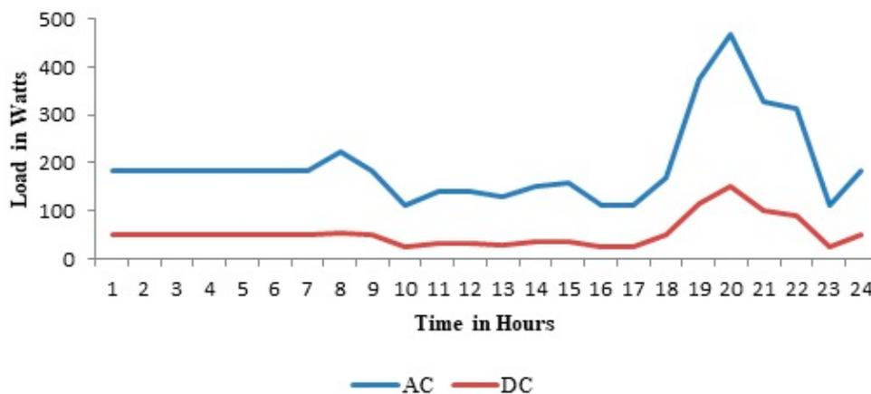
**Figure 4.** Load curve of an individual household with alternating current (AC) and direct current (DC) home appliances.
