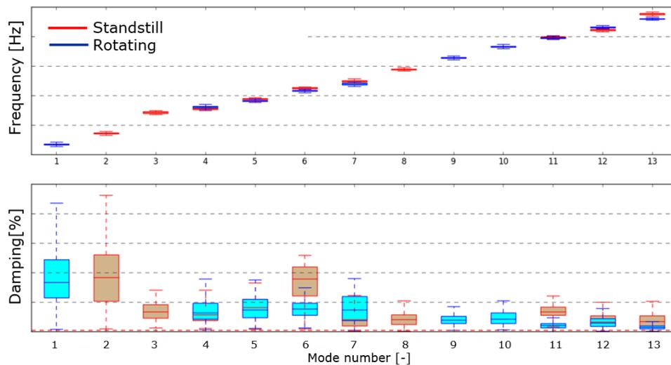
**Figure 11.** Comparison of the tracking procedure applied on data coming from the same machine acquired with the turbine in stand still condition or in normal operating conditions.
