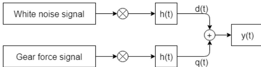
Figure 2. Scheme of the simulated signal.
