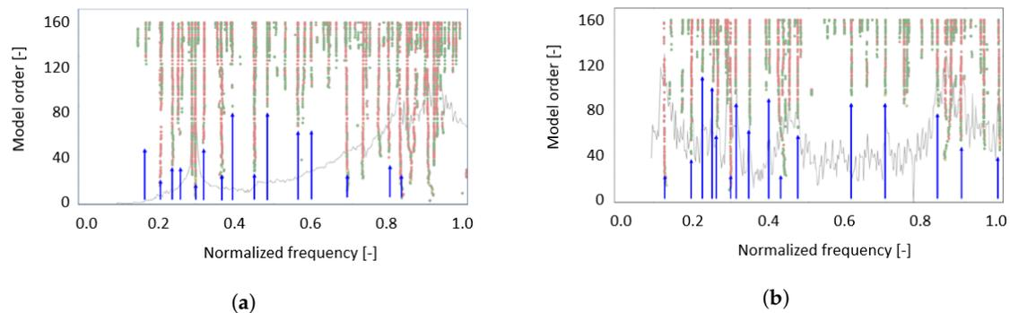
**Figure 8.** Stabilization diagram from a signal taken respectively from the set of data coming from the turbine in idling conditions (a) and from the turbine normally operating (b). Frequency values are normalized for confidentiality reasons.
