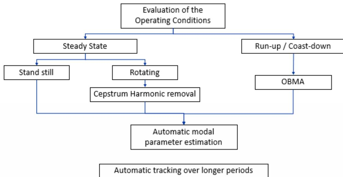
Figure 1. Block diagram of the implemented algorithm.
