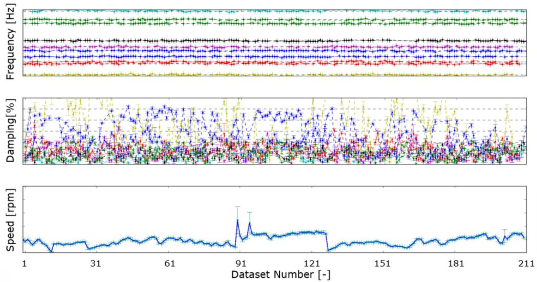
Figure 9. Tracking procedure applied on data sets coming from the machine in stand still conditions.
