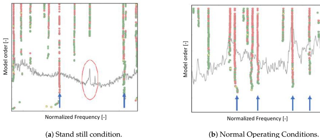
**Figure 12.** Stabilization diagram from a signal taken from the set of data coming from the turbine in stand still conditions (a) and from the turbine normally operating (b). The frequency band is the same for the two figures. Frequency values are normalized for confidentiality reasons.
