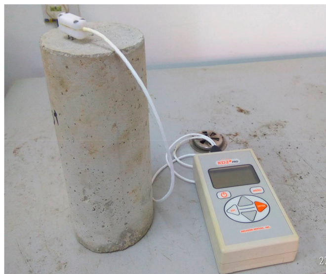
Figure 2. Measurement of thermal properties of mortar using the KD2Pro device.
