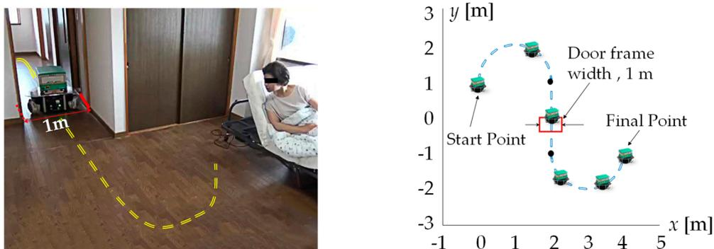
**Figure 15.** One kind of working path in the actual family environment and its setting in two-dimensional coordinates.
