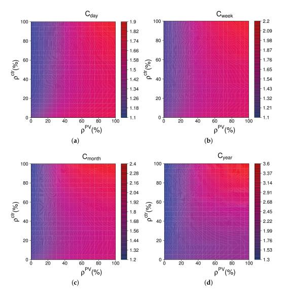
**Figure 4.** Heat map representing the development of the crest factors for different combinations of  $\rho^{PV}$  and  $\rho^{ctr}$  with  $\beta = 0$ : (a)  $\bar{C}_{day}$ ; (b)  $\bar{C}_{week}$ ; (c)  $\bar{C}_{month}$  and (d)  $C_{year}$ .
