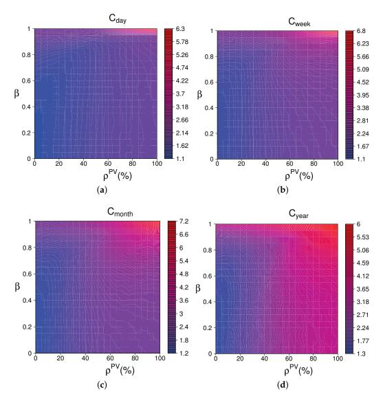
**Figure 3.** Heat map representing the development of the crest factors for different combinations of  $\rho^{PV}$  and  $\beta$  with  $\rho^{ctr} = 100\%$ : (a)  $\bar{C}_{day}$ ; (b)  $\bar{C}_{week}$ ; (c)  $\bar{C}_{month}$  and (d)  $C_{year}$ .
