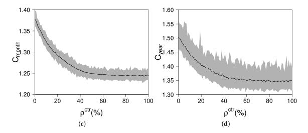
**Figure 2.** Development of the crest factors for different percentages of consumption controlled by the SwarmGrid algorithm. The solid line represents the mean of the crest factors for the 100 simulated seeds. The shaded area is between the maximum and the minimum value obtained from the 100 simulated seeds: (a)  $\bar{C}_{day}$ ; (b)  $\bar{C}_{week}$ ; (c)  $\bar{C}_{month}$  and (d)  $C_{year}$ .
