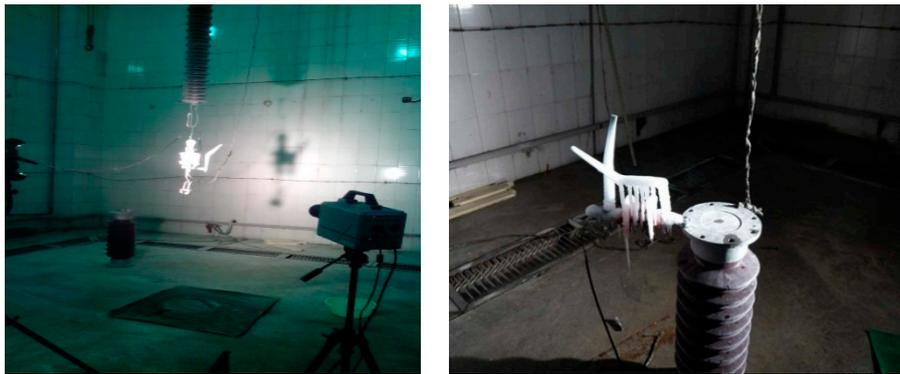
**Figure 4.** Icing withstand voltage test pictures in the UHV DC base of SGCC.
