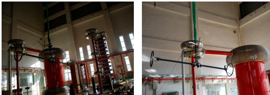
**Figure 3.** Pictures of power frequency discharge voltage testing in the UHV DC base of SGCC.
