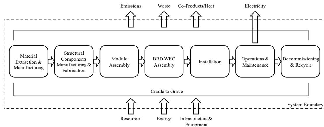
**Figure 2.** Life cycle of BRD WEC and system boundary.
