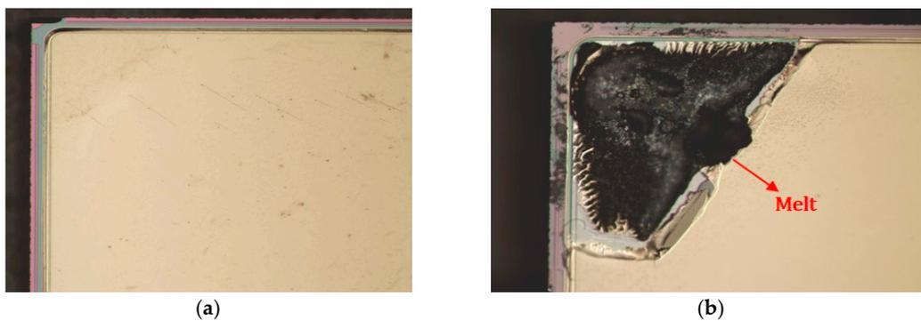
**Figure 9.** Magnified images ( $\times 200$ ) of (a) normal and (b) failed bypass diode.
