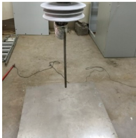
Figure 3. Rod-plane short air gap model layout.
