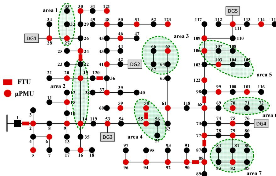
Figure 8. Optimal  $\mu$ PMU placement by IENS.
