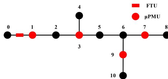
Figure 2. Optimal placement by topological method.
