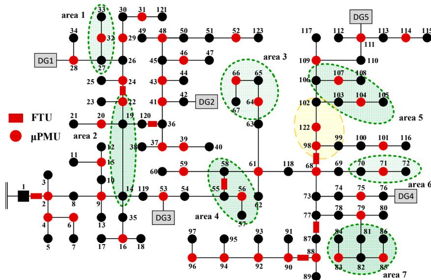
Figure 7. Optimal  $\mu$ PMU placement by topological method.
