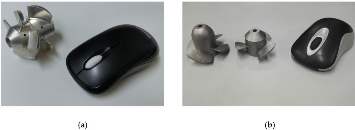
**Figure 1.** The original test turbine and new test turbine of contra-rotating small hydro-turbine. (a) Original test turbine. (b) New test turbine.
