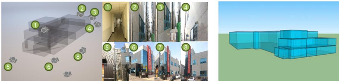
**Figure 7.** Building 3D modeling on testbed 2 using close-range photogrammetry (CRP).
