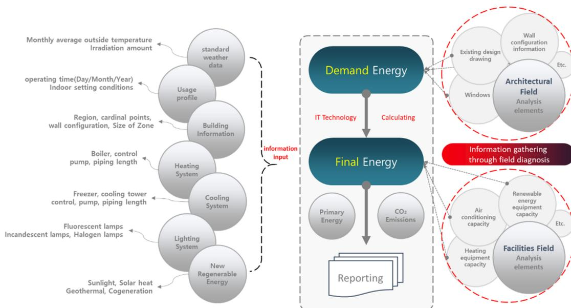
Figure 2. Principle of calculation of energy demand and final energy.
