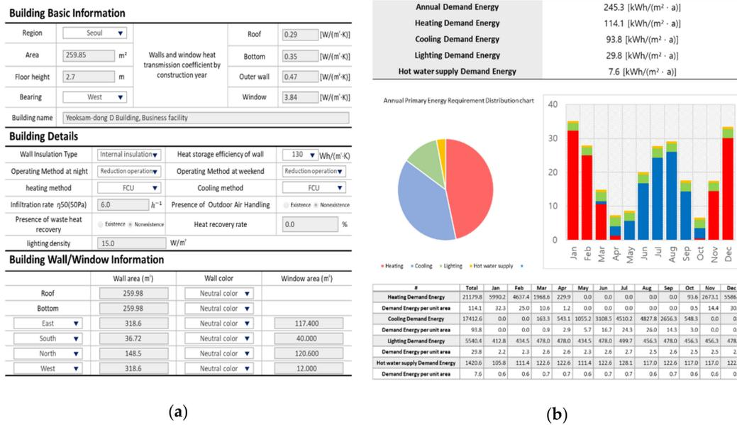
Figure 4. Building-energy performance simulator. UI: analysis of energy demand through diagnosis of the architecture part of testbed 2. (a) Input architecture data of testbed 2; (b) Energy demand.
