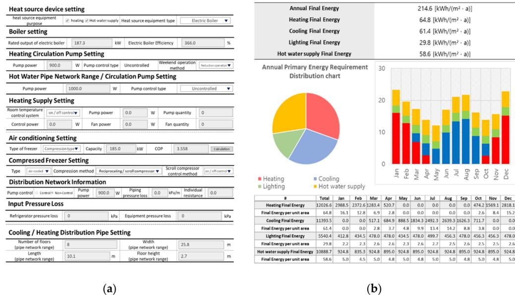
Figure 5. Building-energy performance simulator. UI: analysis of final energy through diagnosis of the facility part of testbed 2. (a) Input facility data of testbed 2; (b) Final energy.
