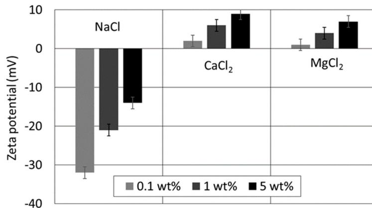
**Figure 2.** Zeta potential of brine/kaolinite with various ion types and concentrations.
