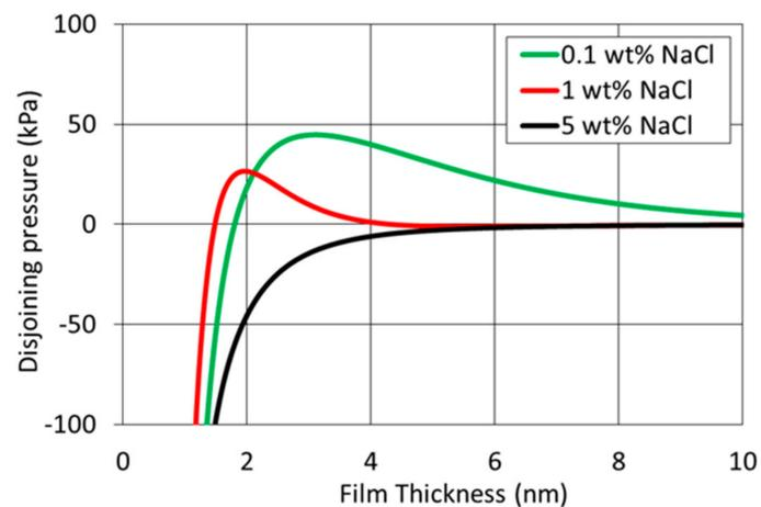
**Figure 4.** Total disjoining pressure, under constant reduced potential, versus interfacial separation of kaolinite and Oil A with presence of various concentration of NaCl.
