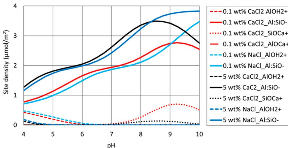
Figure 7. Site density on brine/kaolinite surfaces vs. pH at various ion type and concentration.
