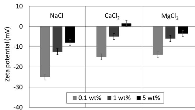
Figure 1. Zeta potential of oil/brine with various ion types and concentrations.
