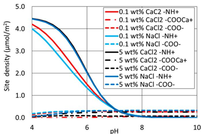
Figure 5. Site density on surfaces of oil/brine vs. pH at various ion type and concentration.
