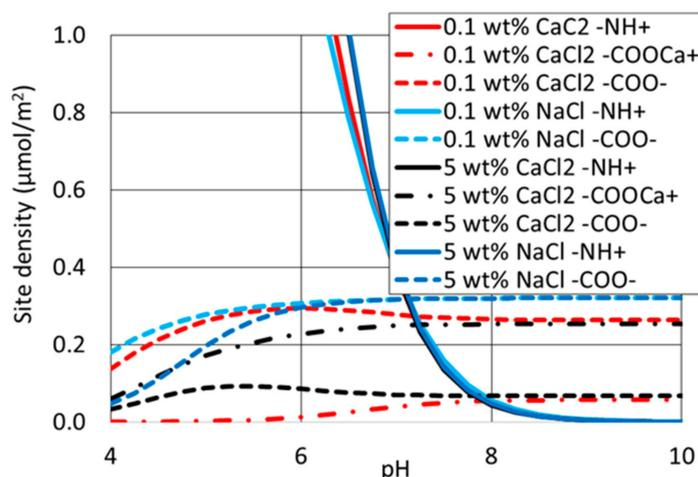
Figure 6. Site density on surfaces of oil/brine vs. pH at various ion type and concentration (this is a plot to particularly observe the site density in a range of 0 to 1  $\mu\text{mol}/\text{m}^2$ ).
