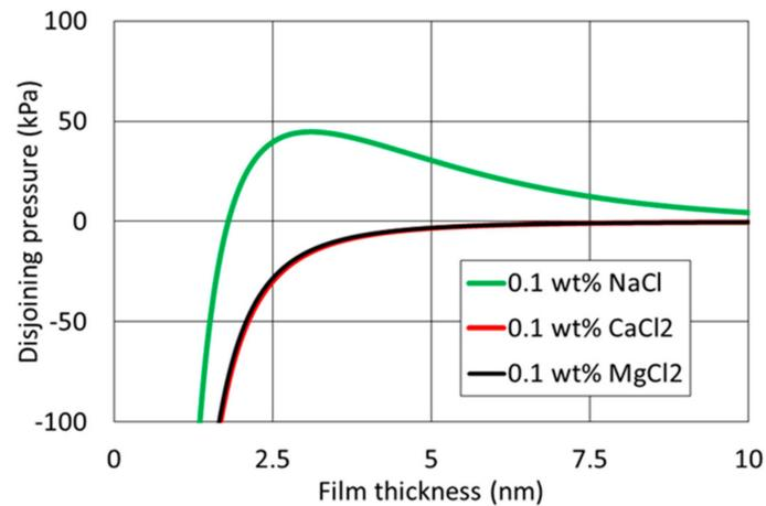
**Figure 3.** Total disjoining pressure, under constant reduced potential, versus interfacial separation of kaolinite and Oil A with presence of various cation types.
