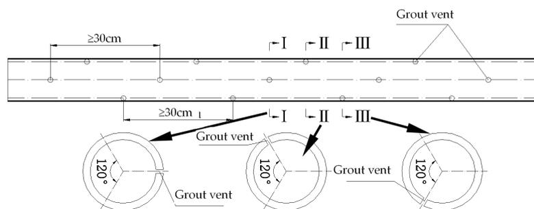
**Figure 5.** Arrangement parameters of grout vents in the body of the casing.
