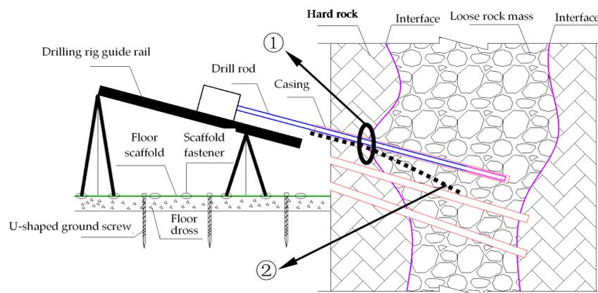
**Figure 3.** Technical difficulties in the process of drilling with casing in the composite rock mass.
