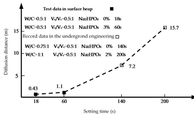
**Figure 7.** Relationship of setting time–vertical diffusion distance of C–S grout in the loose rock mass. W/C: water cement ratio; Vs/Vc: volume ratio of sodium silicate to cement slurry.
