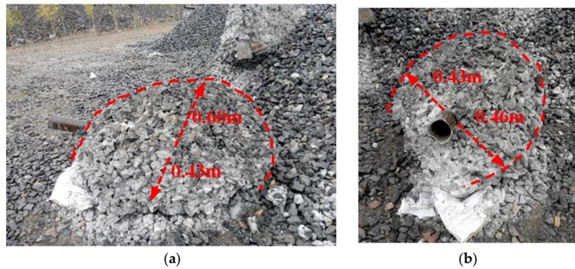
**Figure 6.** Concretion of C–S grout in the seemingly homogeneous loose rock mass (setting time: 18 s): (a) Vertical direction; (b) Horizontal direction.
