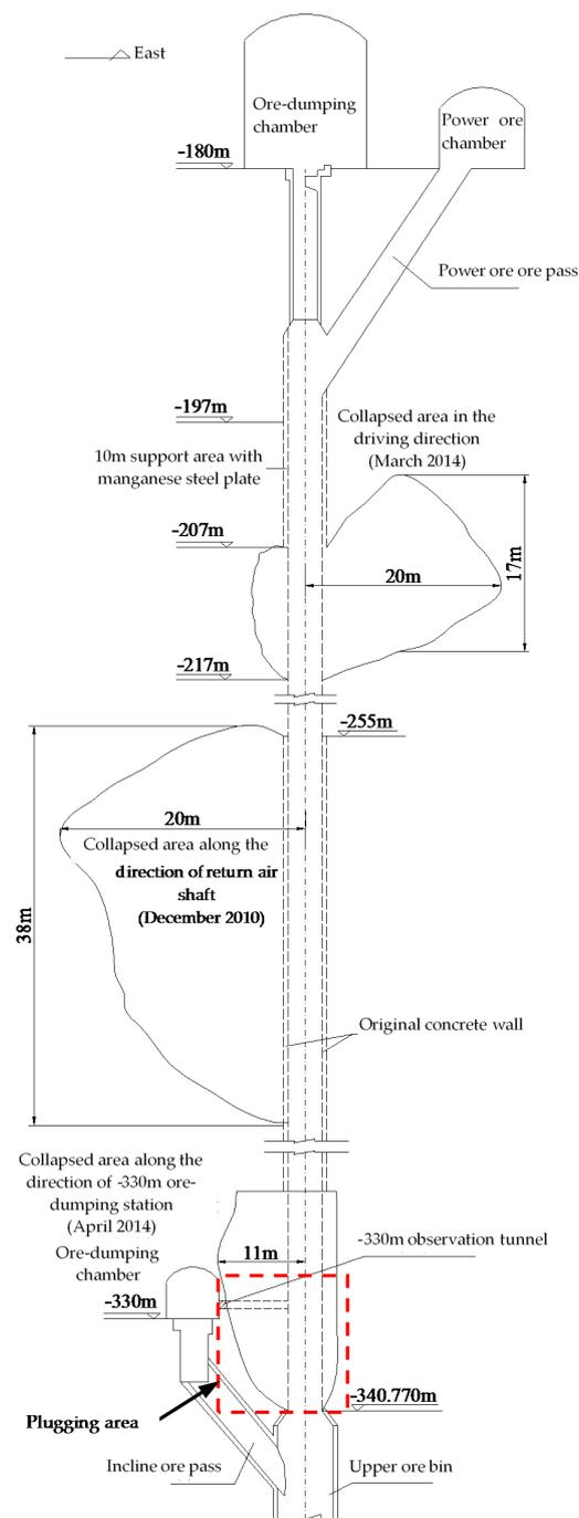
Figure 10. Collapse shapes of the main ore pass.
