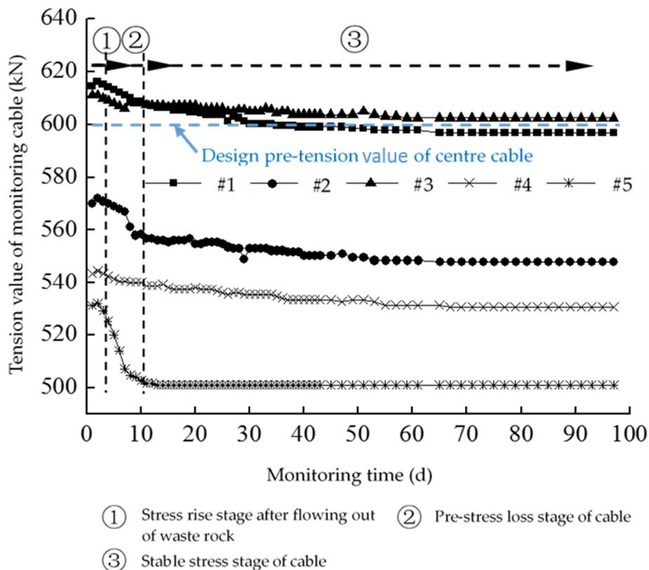
Figure 14. Tension-time curve of monitoring cable.
