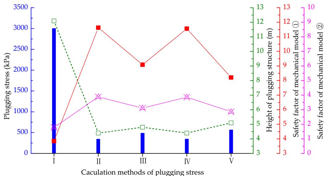
**Figure 11.** The design heights and safety factors of the plugging structure corresponding to different calculation methods of vertical stress.
