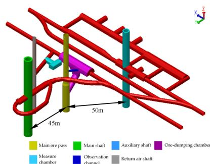
Figure 9. Location plan of the main ore pass.
