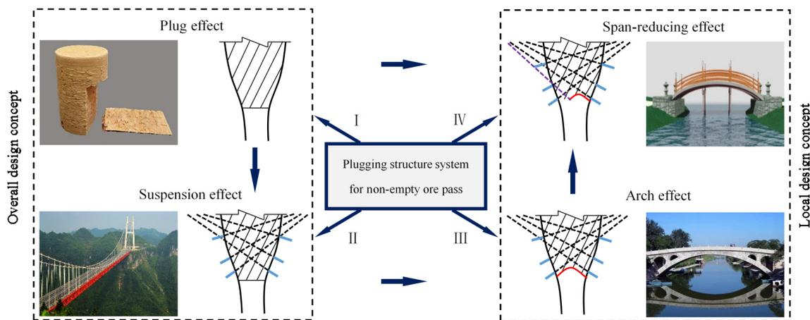
Figure 1. Structure-plugging system for an ore pass in the non-empty condition.
