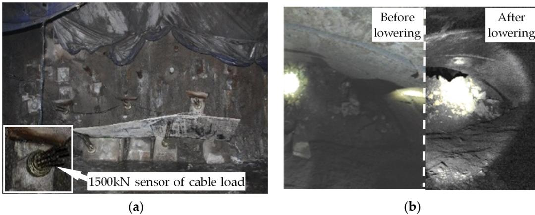
Figure 13. Plugging effect of the main ore pass: (a) Whole picture of plugging engineering; (b) Before and after ore lowering in the incline ore pass.
