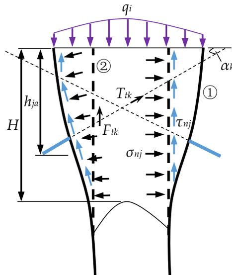
Figure 2. Mechanical models of shear failure of a plugging structure.
