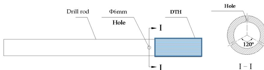
**Figure 4.** Arrangement parameters of holes in the body of the drill rod to prevent sticking. DTH: down-the-hole drill.
