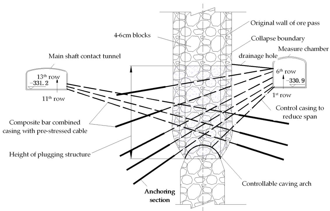
**Figure 12.** Plugging design of the main ore pass.
