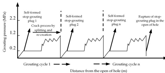
**Figure 8.** Implementation process and method of controllable grouting for inhomogeneous loose rock mass.
