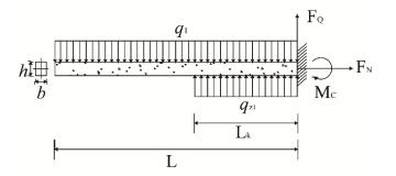
Figure 7. Cantilever structure of KS1.
