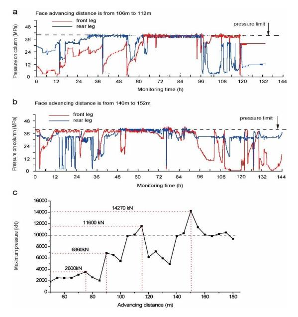
**Figure 13.** Typical mining pressure on the columns and maximum load on support. ((**a**). Mining pressure on column when face advancing from 106 m to 112 m; (**b**). Mining pressure on column when face advancing from 140 m to 152 m; (**c**). Practical maximum pressure on the support in mining process).
