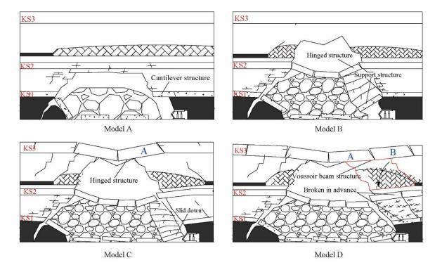
**Figure 6.** Structural models of the overlying strata on the LTCC panel. (Blue part A and B refer to the two key blocks in voussoir beam structure of the key roof strata.).
