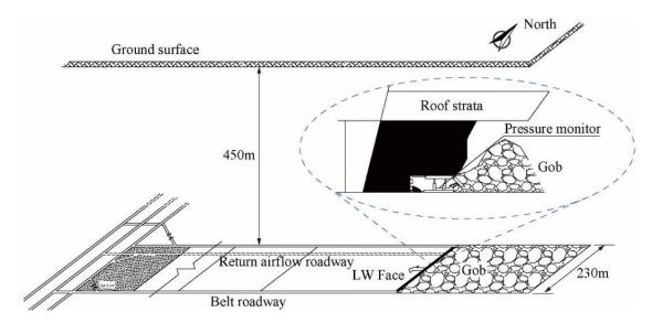
Figure 12. Field measurement diagram in Tashan Coal Mine.
