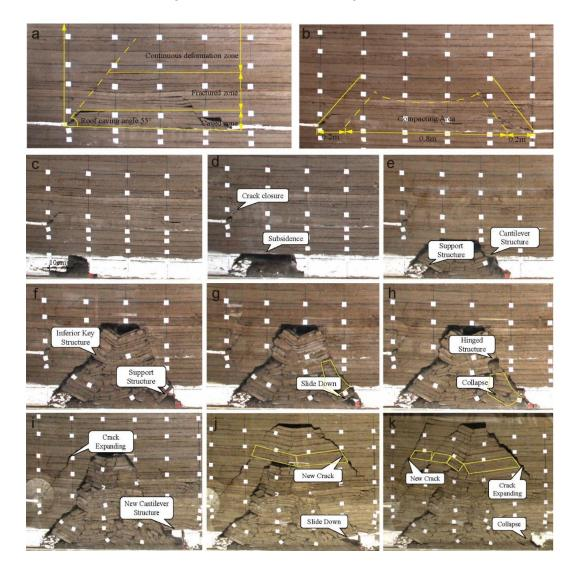
Figure 5. Roof strata behavior of the LTCC panel under an igneous sill and upper gob.
