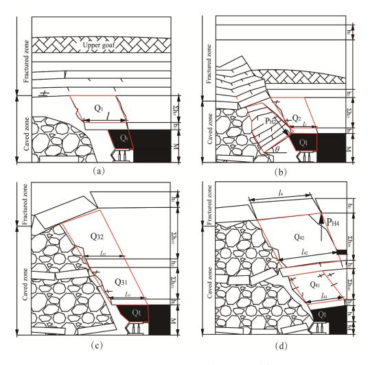
Figure 11. Support resistance calculation models.
