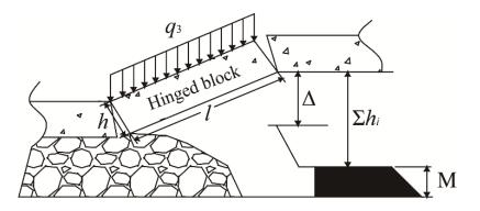
Figure 9. Hinged structure of KS2.
