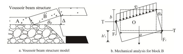
Figure 10. Voussoir structure and mechanical analysis for block B.
