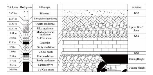
Figure 3. Stratigraphic column of the coal face.
