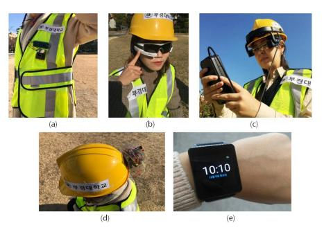
**Figure 5.** Proposed embedded wearable system shown at a mining site: (**a**) sensor-equipped mine safety vest; (**b**) miner wearing Recon Jet Smart Eyewear; (**c**) miner using Epson Moverio BT-2200; (**d**) sensor-equipped safety helmet; (**e**) smartwatch.
