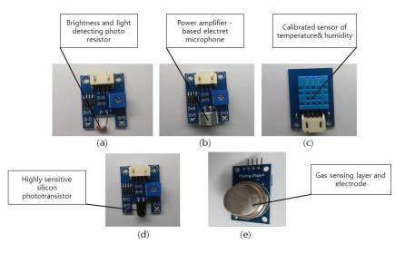
Figure 1. Environmental sensors and their parts: (a) light sensor; (b) sound sensor; (c) humidity sensor; (d) flame sensor; (e) fume sensor.
