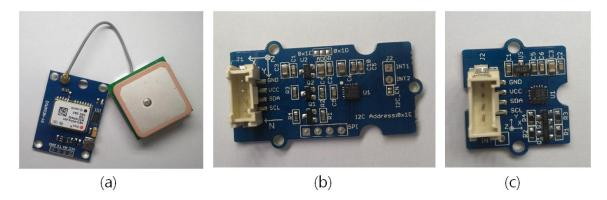
**Figure 3.** Location-tracking sensors: (**a**) global positioning system (GPS) module; (**b**) 6-axis accelerometer and compass; (**c**) digital compass.
