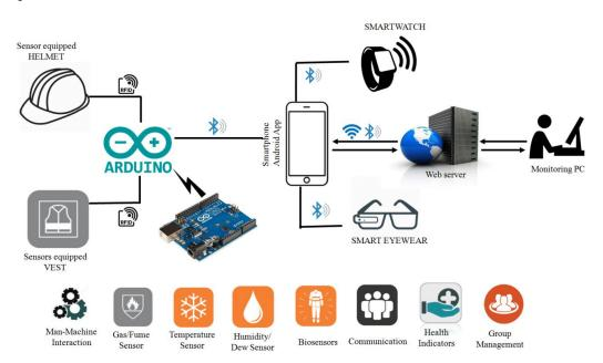
Figure 4. Wearable technology-integrated embedded wearable safety communication system.
