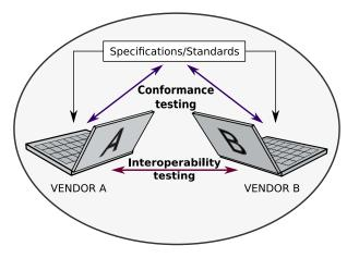
**Figure 16.** Peer-to-peer interoperability testing: independent implementations get connected and their cooperation is evaluated, including verification of exchanged messages (formats and contents).
