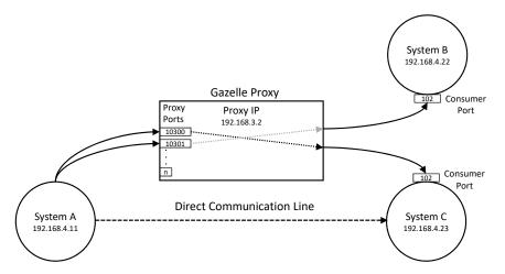
**Figure 17.** Derailing communication via Gazelle proxy service: port numbers are assigned to the systems prior testing, transferred messages are captured to undergo validation.
