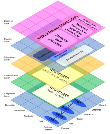
**Figure 9.** Positioning of features in the three-dimensional SGAM: selected VPP features mapped onto the three reference designation axes.
