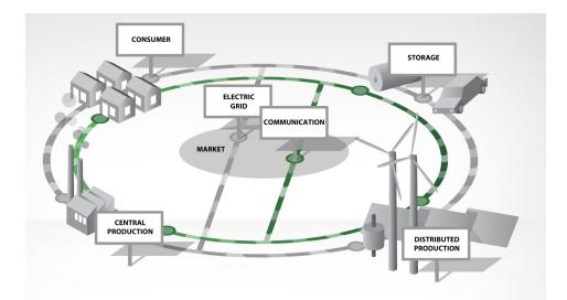
**Figure 1.** The Smart Grid: Services based on Information and Communication Technology (ICT) are added to the established energy management paradigm to support efficient grid control in the presence of distributed energy resources (DER).
