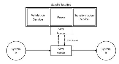
**Figure 18.** Schematic set-up for interoperability testing: directional communication is routed through the VPN connection to capture, transform and validate messages using the according Gazelle tools.
