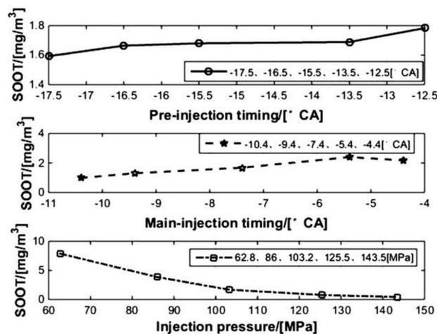
Figure 7. Effects of different injection parameters on soot emissions.
