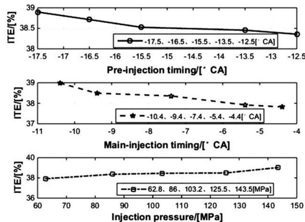
Figure 8. Effects of different injection parameters on efficiency.
