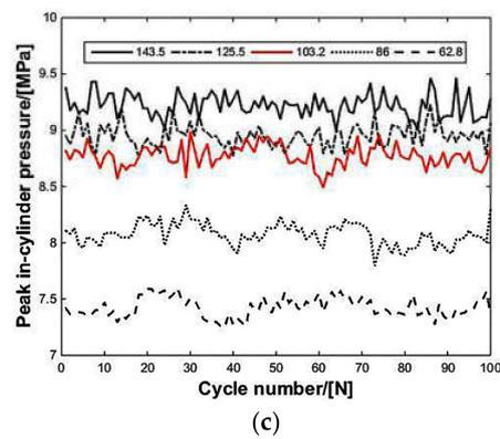
**Figure 4.** Effects of different injection parameters on the combustion stability. (a) Different pre-injection timings; (b) Different main-injection timings; (c) Different injection pressure
