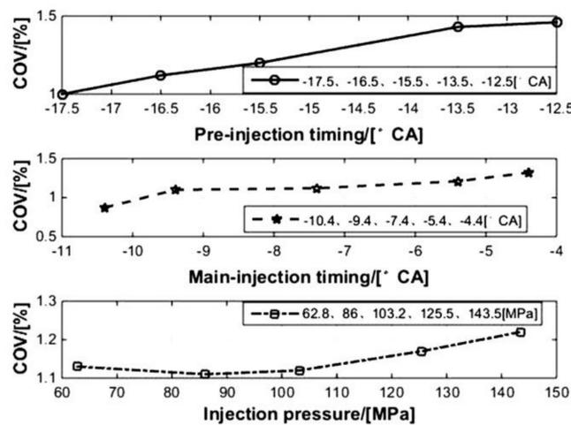
**Figure 5.** Effects of different injection parameters on the coefficient variation (COV).
