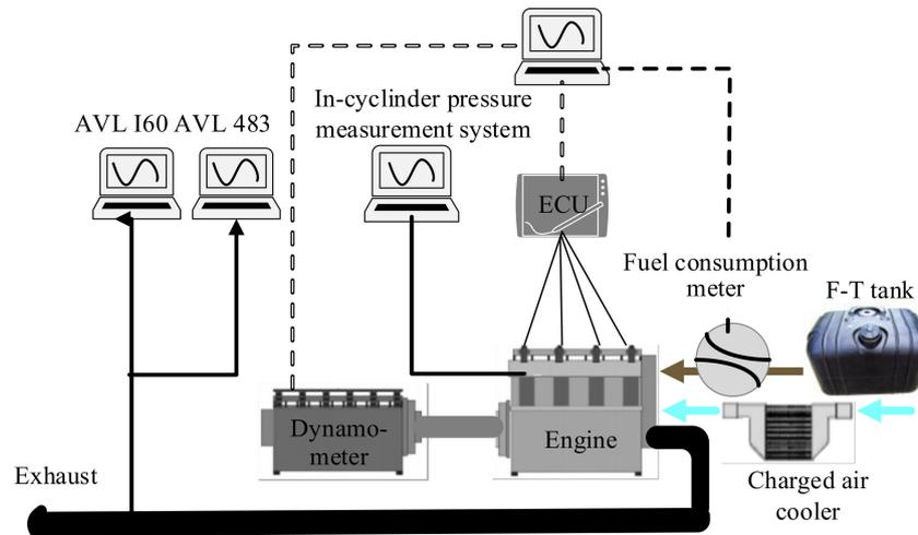
**Figure 1.** Test bench setup. ECU: Electronic Control Unit; F-T: Fischer-Tropsch**Table 2.** Accuracy and uncertainty of the measuring equipment. F-T: Fischer-Tropsch.
