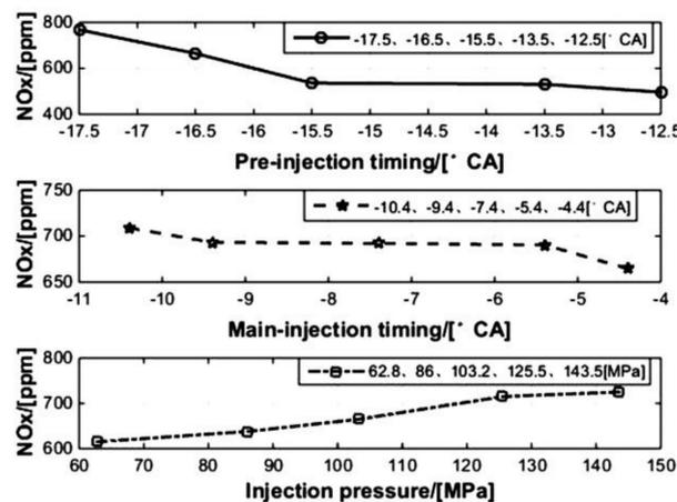
Figure 6. Effects of different injection parameters on NO<sub>x</sub> emissions.
