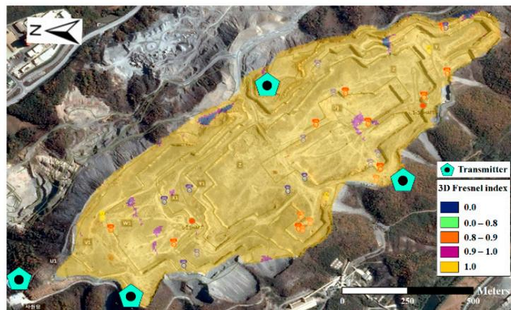
Figure 14. 3D Fresnel index overlay map for the four transmitters in the open-pit mine.
