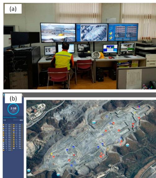
**Figure 13.** An open-pit mine in South Korea with a wireless communications system for fleet management of mine equipment. (a) Control center. (b) Main dashboard.
