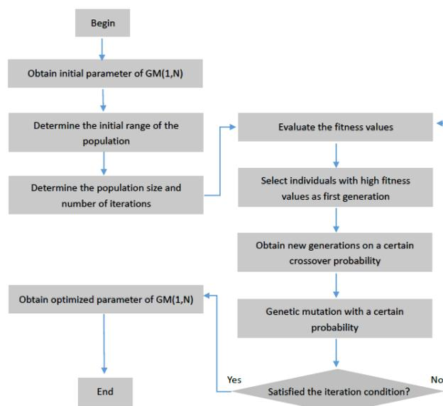
**Figure 1.** The flow chart of the GM(1,N) model optimized using a genetic algorithm.
