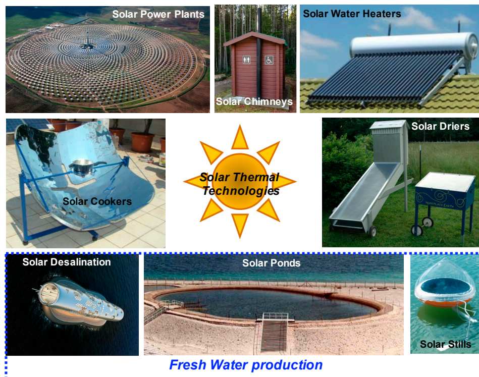
Figure 1. The present solar thermal technologies under the sunlight irradiance include, but not limited to the solar power plants [23], solar chimneys [24], solar water heaters [25], solar cookers [26], solar driers [27], solar desalination [28], solar ponds [29], and solar stills [30]. The latter three technologies are used to produce fresh water. Images reproduced from the corresponding web links.
