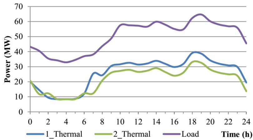
Figure 4. Thermal diagram comparison with load diagram.
