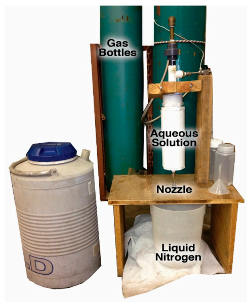
Figure 7. Apparatus used to generate THF and TBAB hydrate crystals.
