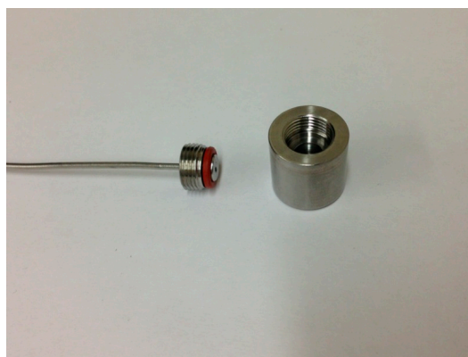
Figure 2. Photograph of the MCDSC high pressure sample cell and closure.
