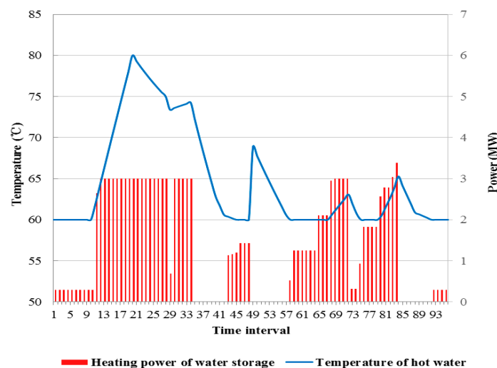
Figure 10. Heating power of the water storage tank and the temperature of hot water on a typical winter day.
