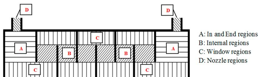
Figure 1. Pressure drop regions in a shell and tube heat exchanger.
