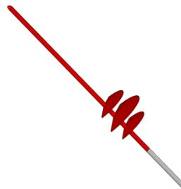
Figure 1. The high voltage end simplified model of composite insulator.
