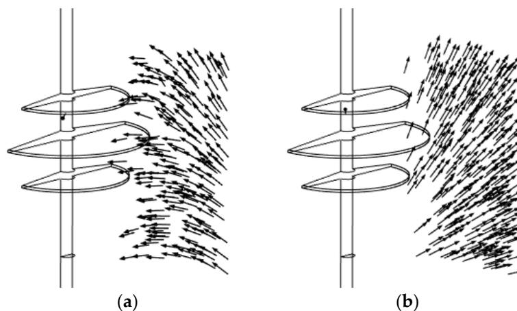
**Figure 7.** The direction map of (a) air drag force and (b) electric force on particles at 0.28 s after release.
