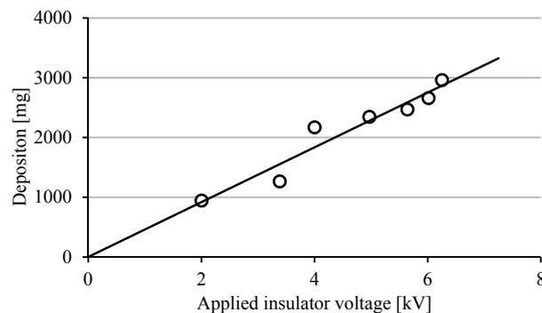
**Figure 10.** The relationship between deposition and applied insulator voltage [33].
