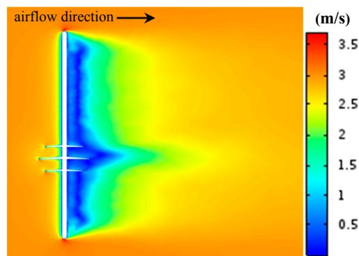
**Figure 3.** The contour map of airflow velocity in the insulator axial section.
