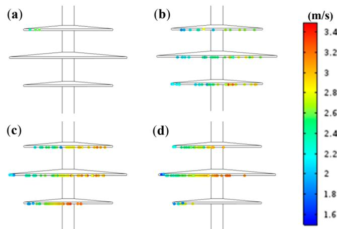
**Figure 5.** The distribution map of contamination particles frozen on insulator surface, when (a)  $Q = 1$  p.u.; (b)  $Q = 10$  p.u.; (c)  $Q = 30$  p.u.; and (d)  $Q = 50$  p.u.
