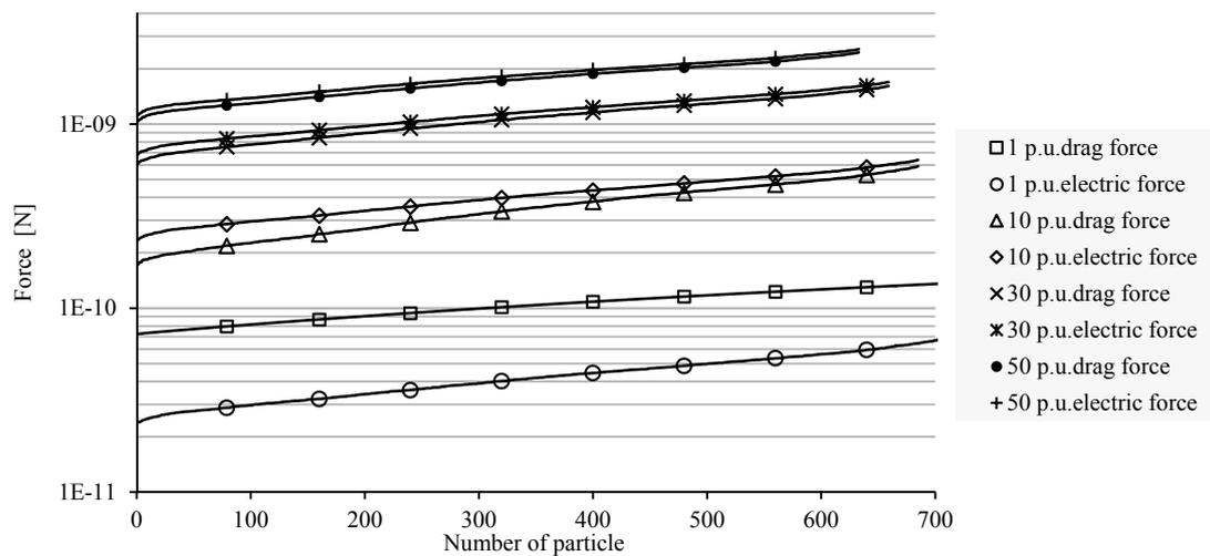
**Figure 8.** The curves of drag force and electric field force on the particles with different  $Q$ .
