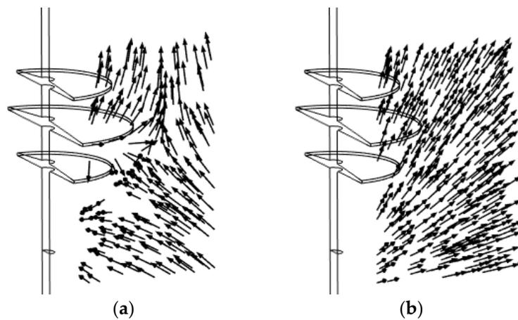
**Figure 6.** The direction map of (a) air drag force and (b) electric force on particles at 0.19 s after release.
