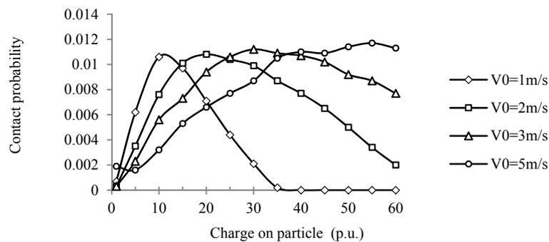
**Figure 9.** The relationship of electric charge on particles and particles contact probability with different airflow velocity  $V_0$ .
