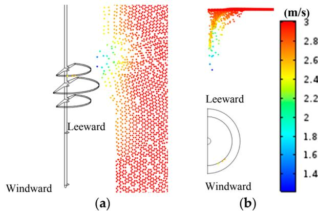
**Figure 4.** The map of contamination particles movement position from (a) aerial view and (b) top view after being released for 0.4 s.
