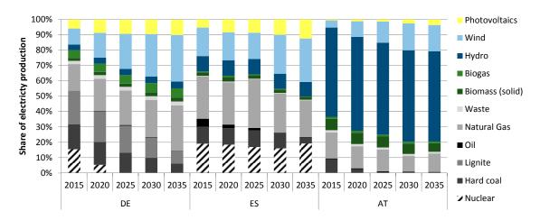
Figure 2. Projected structural change of electricity mixes in Austria, Spain and Germany.
