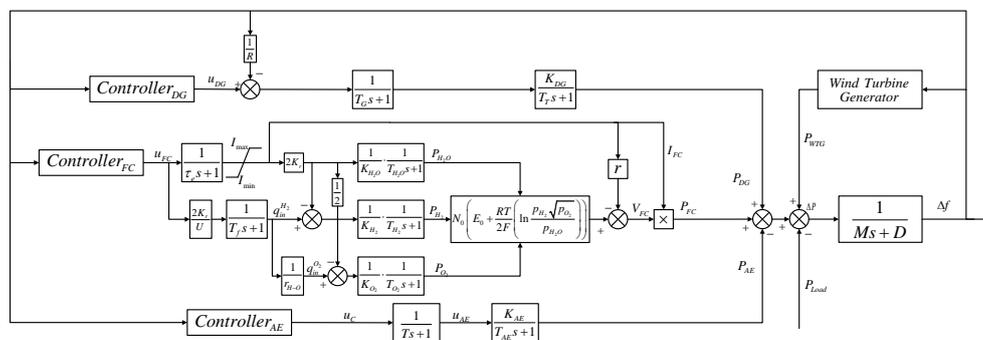
**Figure 8.** Microgrid power system control strategy.
