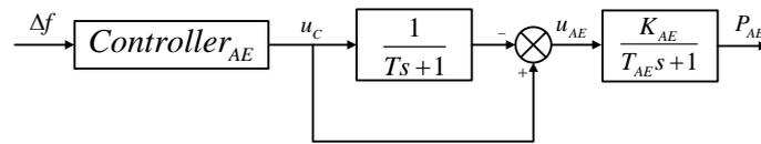
Figure 6. Aqua Electrolyzer Supplementary Control Block.
