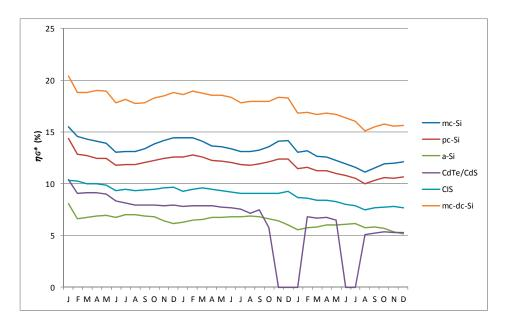
Figure 15. Evolution of the operating PV generators efficiency.
