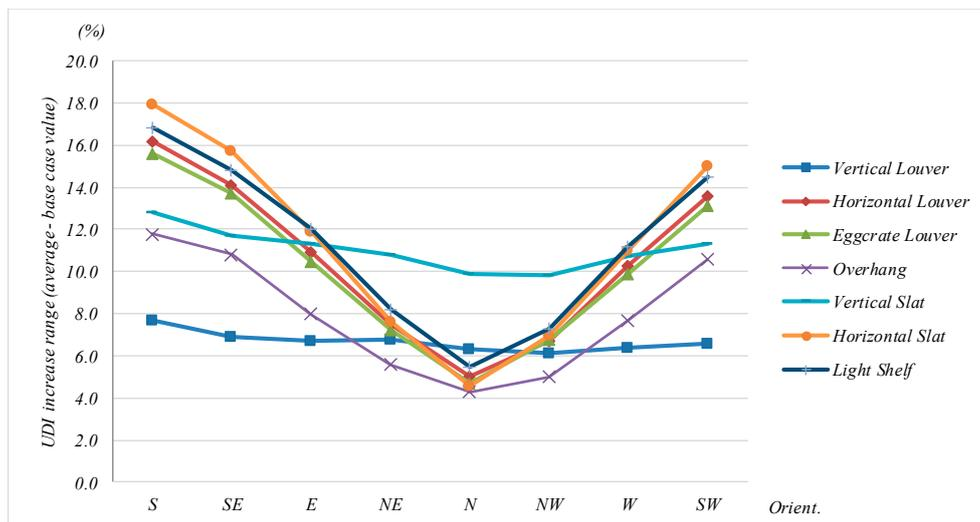
Figure 19. UDI value increase range (the differences between the baseline and average values) comparison by façade shading type.
