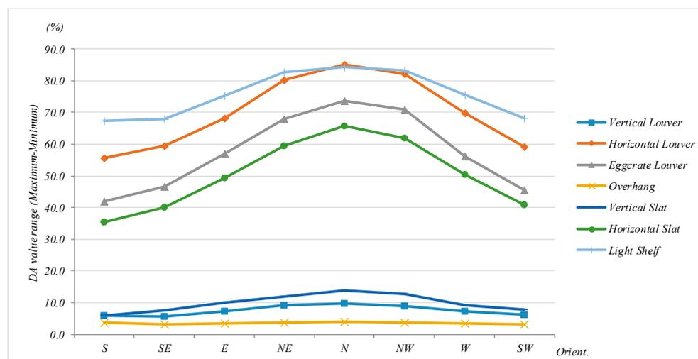
**Figure 20.** DA value range (the differences between the maximum and minimum values) comparison by façade shading type.
