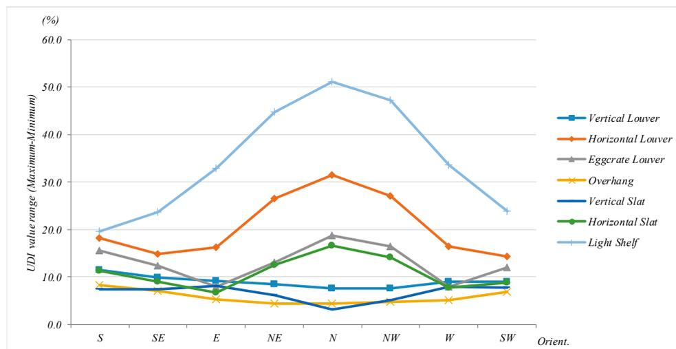
**Figure 21.** UDI value range (the differences between the maximum and minimum values) comparison by façade shading type.
