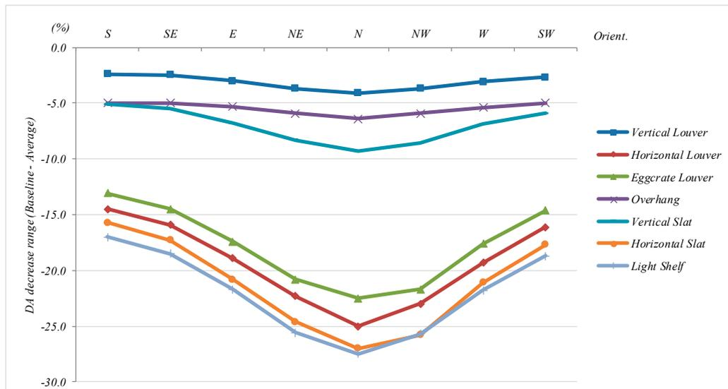
Figure 18. DA value decrease range (the differences between the average and baseline values) comparison by façade shading type.
