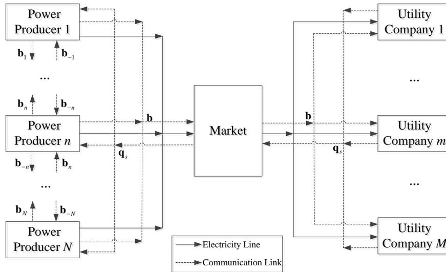
Figure 1. Generation side bidding transaction model.
